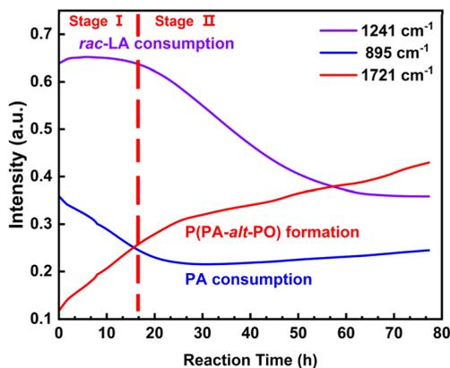
Fig. 5 Time-resolved *in situ* IR spectra during the polymerization of mixtures of PA, PO, and *rac*-LA. Reaction conditions: CHD/(*S,S*)-TUC/PA/PO/*rac*-LA = 1/5/100/200/200,  $80^\circ\text{C}$ , and toluene as the solvent.
