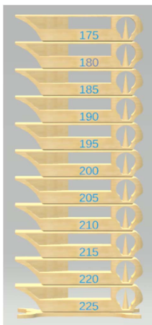
Fig. 1 Design photo of the calibration tower.
