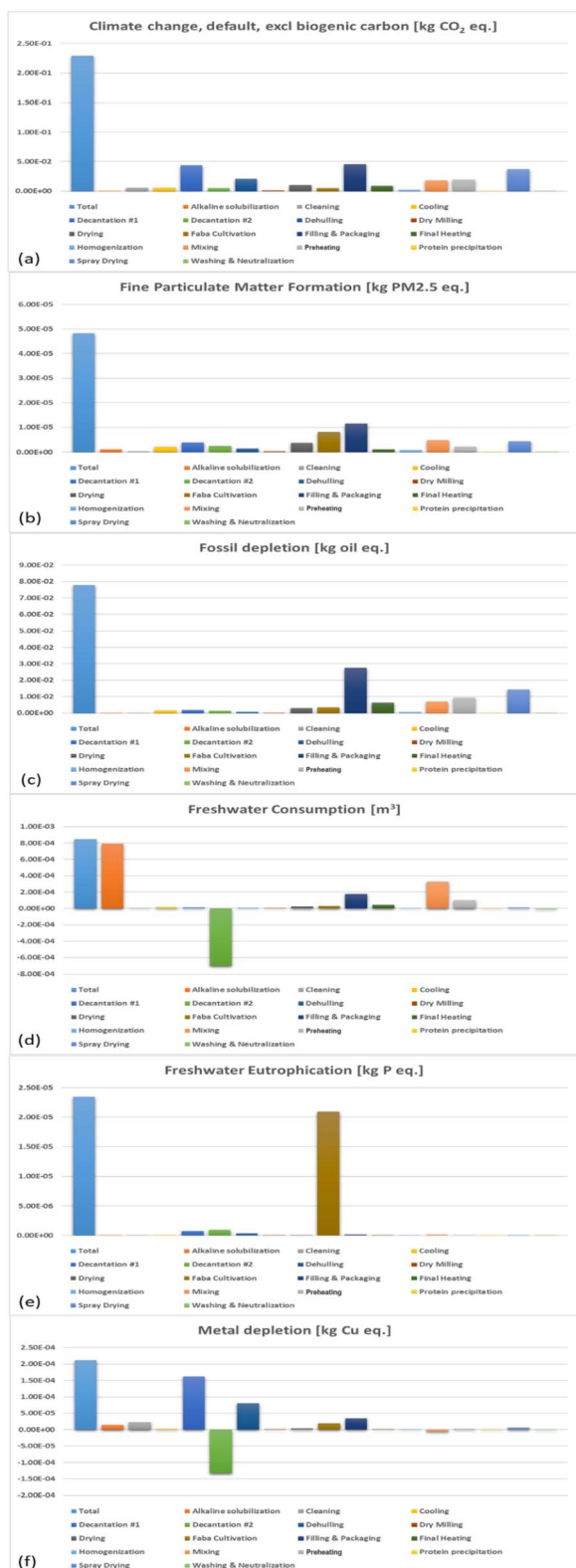
Fig. 2 Environmental impact of the beverage production on (a) climate change (kg CO 2 eq.), (b) fine particulate matter formation (kg PM 2.5 eq.), (c) fossil depletion (kg oil eq.), (d) freshwater consumption (m 3 ), (e) freshwater eutrophication (kg P eq.) and (f) metal depletion (kg Cu eq.).
