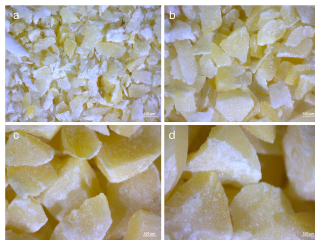
Fig. 1 Microscope images of the distinct particle size fractions of the ground peas used in this work: (a) small ( 0.25 \text{ mm} \leq x < 0.5 \text{ mm} ), (b) medium ( 0.5 \text{ mm} \leq x < 1 \text{ mm} ), (c) large ( 1 \text{ mm} \leq x < 2 \text{ mm} ), and (d) extra-large ( 2 \text{ mm} \leq x < 3.15 \text{ mm} ).
