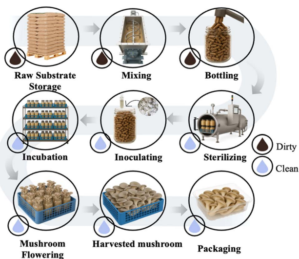
Fig. 1 Processing steps for producing mushrooms. Densified biomass pellets used as the substrate are first stored on pallets, then mixed in a ribbon blender, and finally filled into jars. These jars undergo steam sterilization before being inoculated with either solid or liquid spawn. Following inoculation, the jars are incubated to allow mycelial colonization, which eventually leads to the formation of mushroom fruiting bodies. The mature mushrooms are then harvested, packaged, and distributed. Brown and blue droplets represent dirty and clean steps, respectively, highlighting the importance of maintaining a sanitary flow throughout the process.
