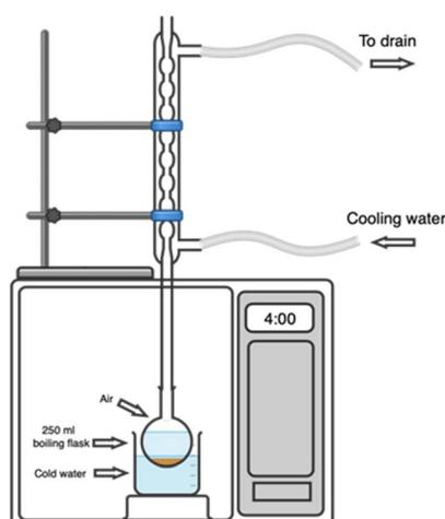
Fig. 1 Modified microwave oven for microwave-assisted extraction (MAE).
