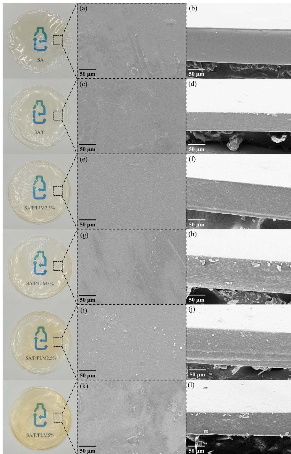
Fig. 1 Photographs of the films (left) and micrographs of the surfaces and cross-sections at 1000 $\times$  magnification (right) of the films SA (a and b), SA/P (c and d), SA/P/LIM2.5% (e and f), SA/P/LIM5% (g and h), SA/P/PLM2.5% (i and j), and SA/P/PLM5% (k and l).
