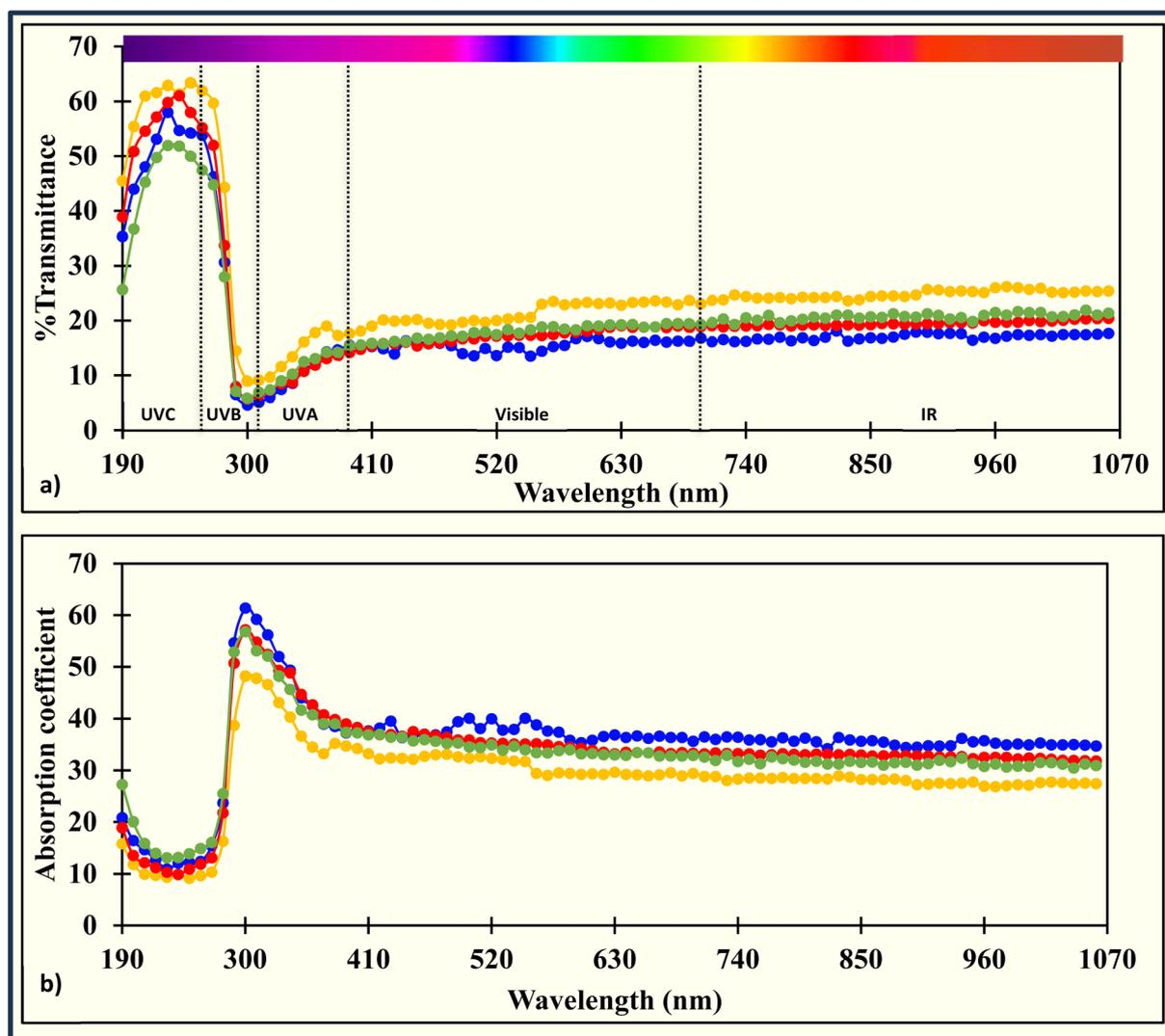
**Fig. 4** Film's (a) % transmittance and (b) absorption coefficient of the electromagnetic radiation throughout the UV-Vis-IR region. Yellow, blue, red, and green lines are given for ACR (yellow line), ACR-ι1.5% (blue line), ACR-κ1.5% (red line), and ACR-λ1.5% (green line) films, respectively. The addition of carrageenan has significantly improved the light-blocking capability of films.
