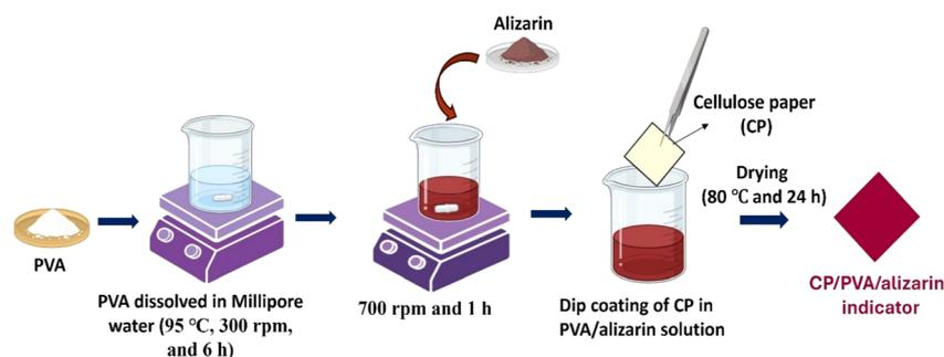
Fig. 1 Schematic depicting the fabrication of CP/PVA/alizarin indicator.
