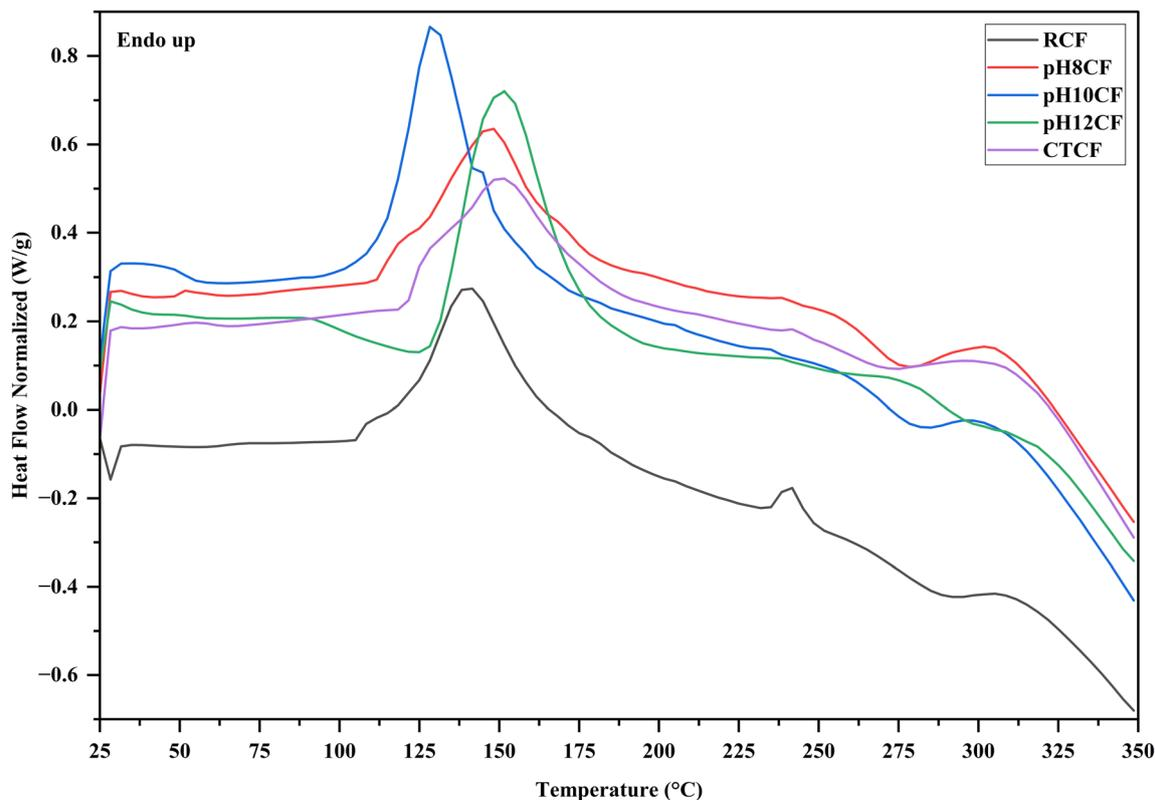
Fig. 11 Thermal analysis of RCF and modified CFs.
