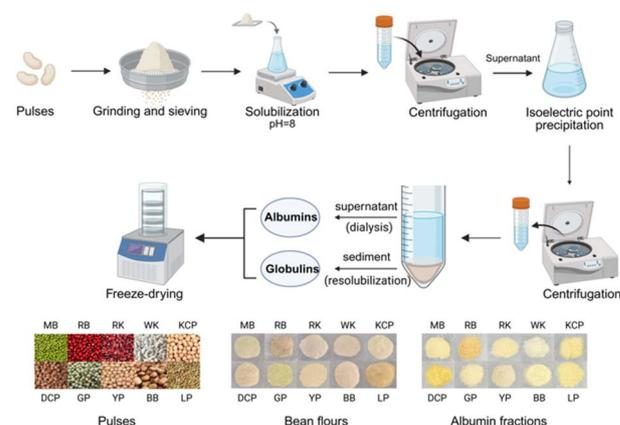
Fig. 1 A schematic overview of the pulse protein extraction process.
