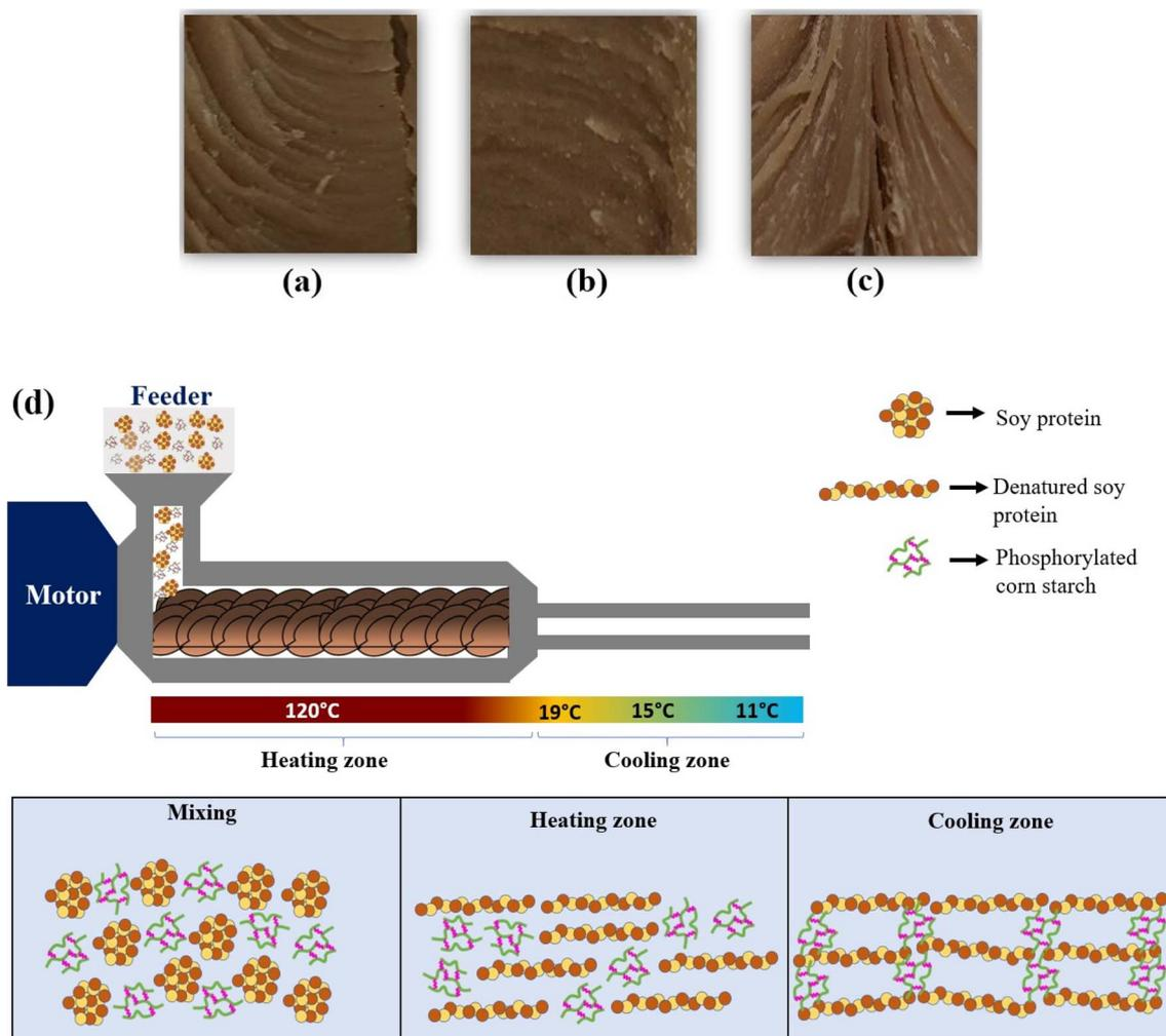
Fig. 8 (a) HMMAs from SPI–NCS (80 : 20) showing a moderate fibrous structure. (b) SPI–PCS (0.04%  $\text{POCl}_3$ , 80 : 20) showing less fiber formation. (c) SPI–PCS (0.01%  $\text{POCl}_3$ , 80 : 20) with a distinct, thin fibrous structure. (d) Schematic illustration of the hypothesised mechanism.
