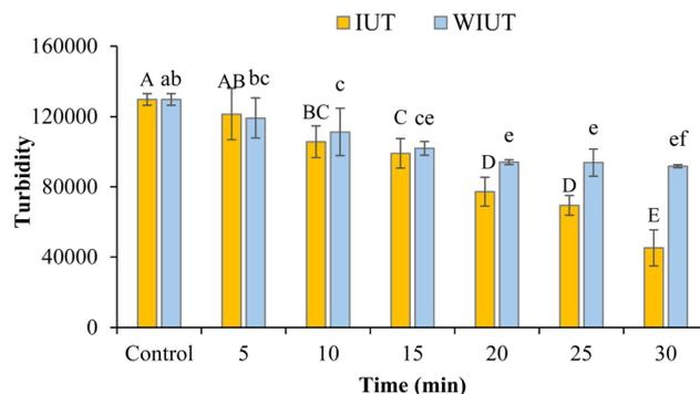
Fig. 1 Turbidity of FBP-oil emulsions at different US-treatment times and treatment conditions (IUT and WIUT). Different uppercase and lowercase superscripts indicate significant differences ( $p < 0.05$ ) for the IUT and WIUT samples, respectively.
