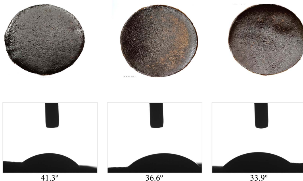
Fig. 9 Contact angle of biocomposites reinforced with plant fibres.
