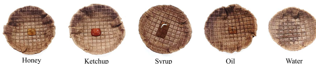
Fig. 11 Spreadability test of the biodegradable plates with different food models within 15 min.
