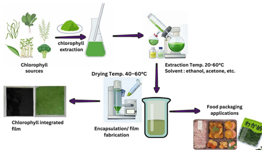
Fig. 2 Schematic of chlorophyll-based active film synthesis. 46,47
