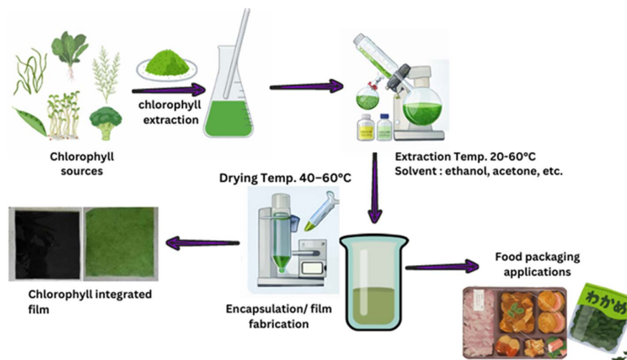
Fig. 2 Schematic of chlorophyll-based active film synthesis. 46,47
