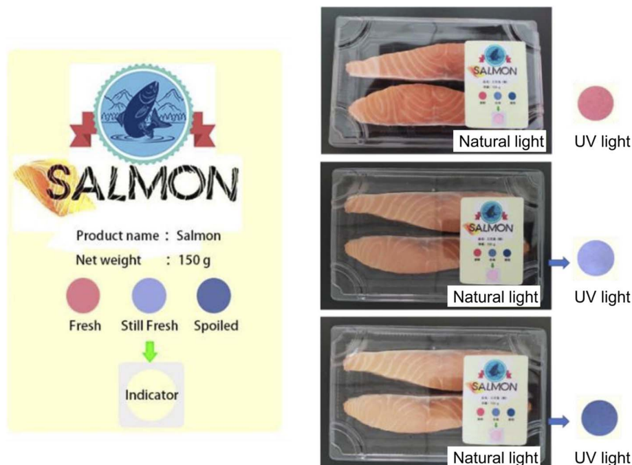
Fig. 2 Schematic layout of the sensing label (left) and demonstration of its application in salmon samples (right). Reproduced from ref. 107 with permission from Elsevier B.V.
