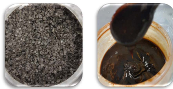
Fig. 3 Samples of sorted side streams of skin and viscera of seabream and seabass after stabilization with a patented dehydration procedure (DFS and DFV). From left to right: dehydrated fish skin (DFS), exhibiting a solid texture, and dehydrated fish viscera (DFV), exhibiting an oily/creamy texture (see Table 2).
