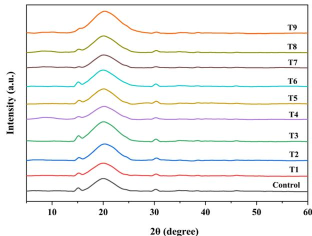
Fig. 4 X-ray diffraction patterns of control and cold plasma-treated chia seed flour samples.
