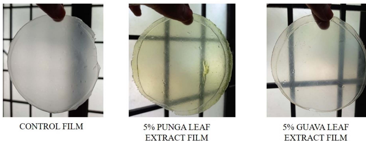
Fig. 6 Preparation of bioactive films with varying concentrations of leaf extracts.
