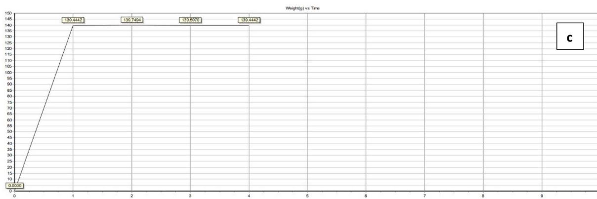
Fig. 8 Water vapor transmission rate (WVTR) of control and extract-based starch films – (a) control film; (b) P. pinnata leaf extract incorporated film; (c) P. guajava leaf extract incorporated film.
