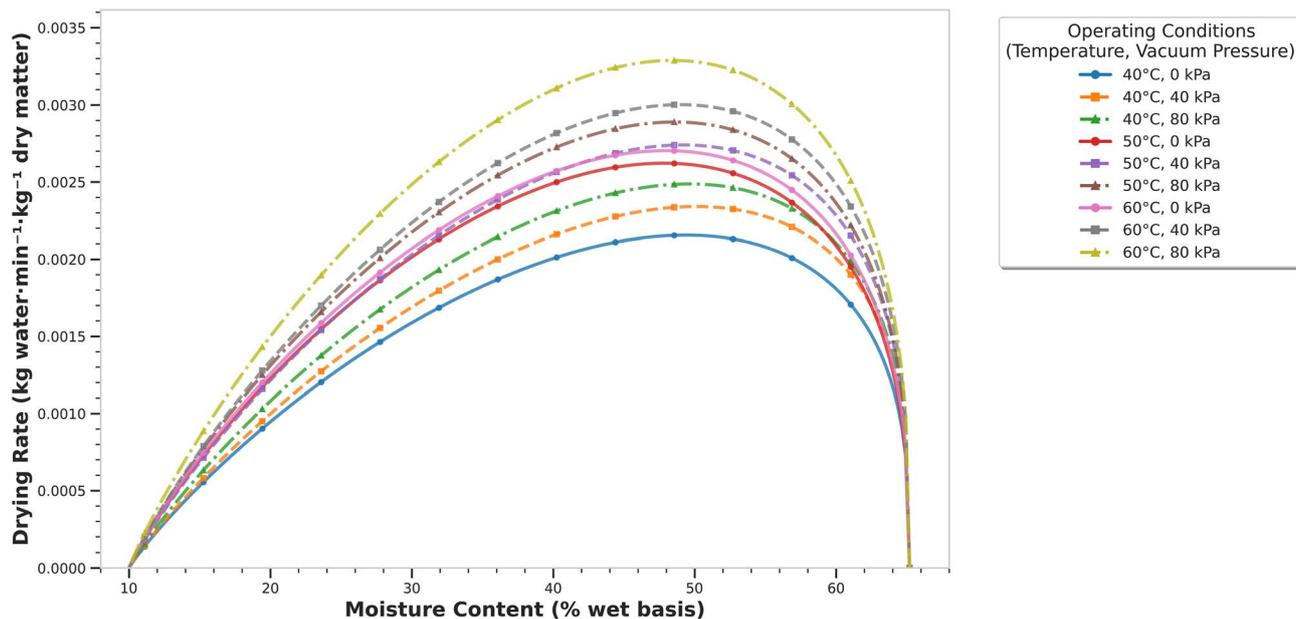
Fig. 2 Drying performance under different operating conditions.
