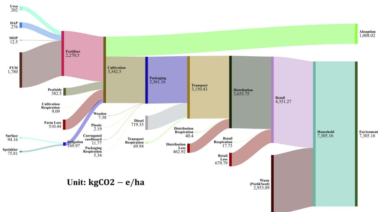
Fig. 3 Detailed diagram illustrating CO<sub>2</sub>-e emissions and losses across the litchi supply chain.
