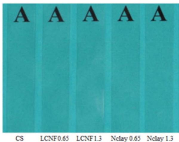
Fig. 6 Visual appearance of films based on cassava starch (CS), CS with lignocellulosic nanofibers (LCNF) and nanoclay (Nclay). Reproduced from Travalini *et al.*, 2019.<sup>76</sup> Copyright Elsevier 2019.
