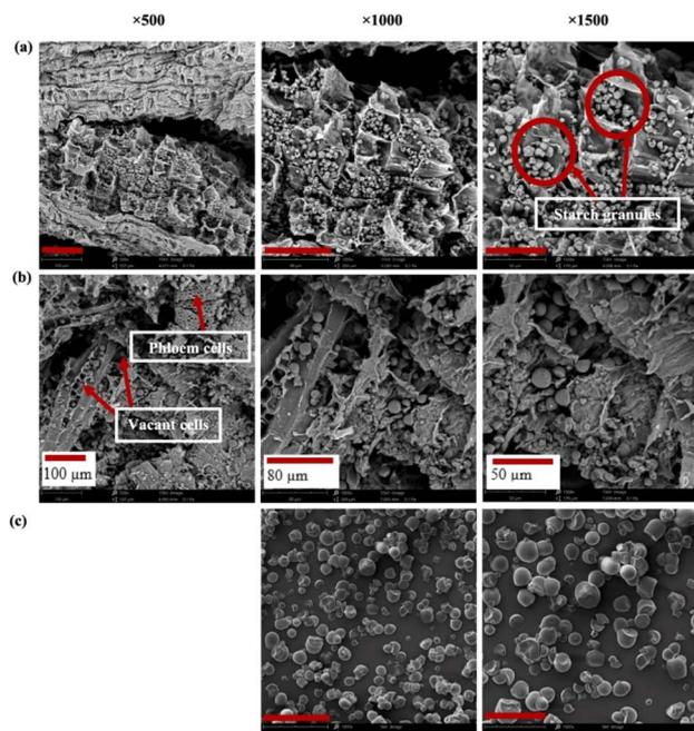
Fig. 3 Scanning electron microscope micrographs representing the surface morphology of (a) cassava peel, (b) cassava bagasse, and (c) commercial cassava starch. Reproduced from Thuppahige *et al.*, 2023.<sup>44</sup> Copyright Elsevier 2023.
