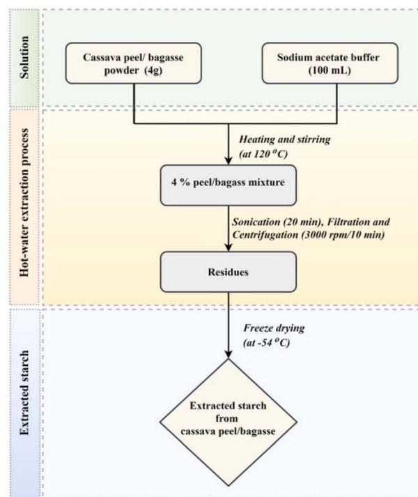
Fig. 5 Extraction of starch via hot water extraction using cassava peel and cassava bagasse. Reproduced from Thuppahige *et al.*, 2023.<sup>56</sup> Copyright Elsevier 2023.
