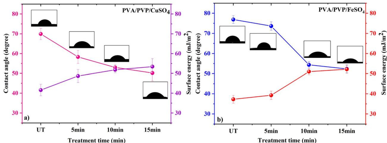
Fig. 3 Contact angle analysis of (a) PVA/PVP/CuSO<sub>4</sub> and (b) PVA/PVP/FeSO<sub>4</sub> polymer films.
