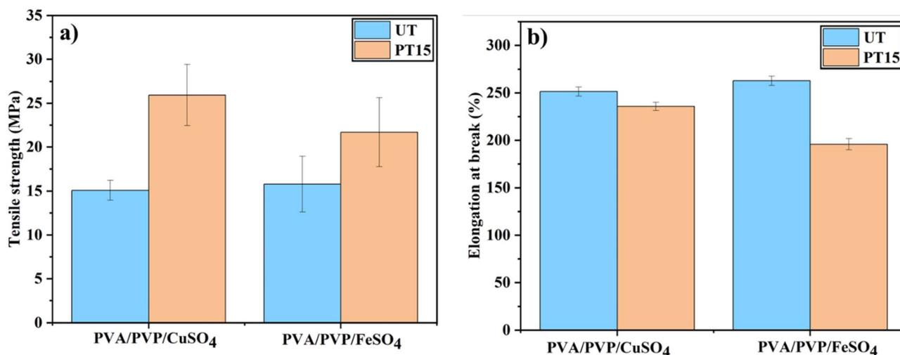
Fig. 10 (a) Tensile strength and (b) elongation at break of PVA/PVP/ $\text{CuSO}_4$  and PVA/PVP/ $\text{FeSO}_4$  polymer films.
