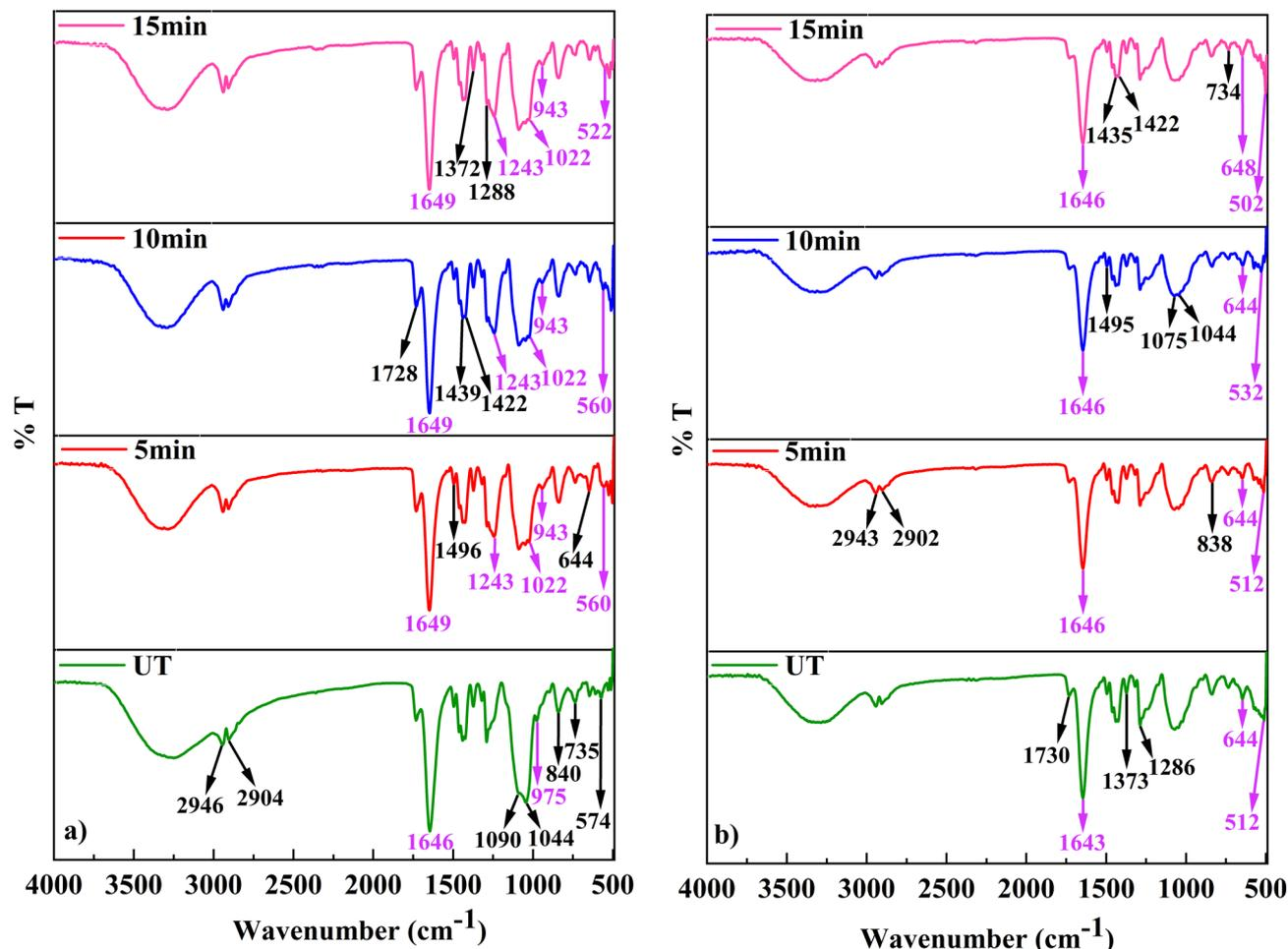
Fig. 5 FTIR analysis of (a) PVA/PVP/CuSO<sub>4</sub> and (b) PVA/PVP/FeSO<sub>4</sub> polymer films.
