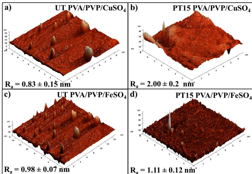
Fig. 8 AFM analysis of PVA/PVP/CuSO<sub>4</sub> and PVA/PVP/FeSO<sub>4</sub> polymer films.
