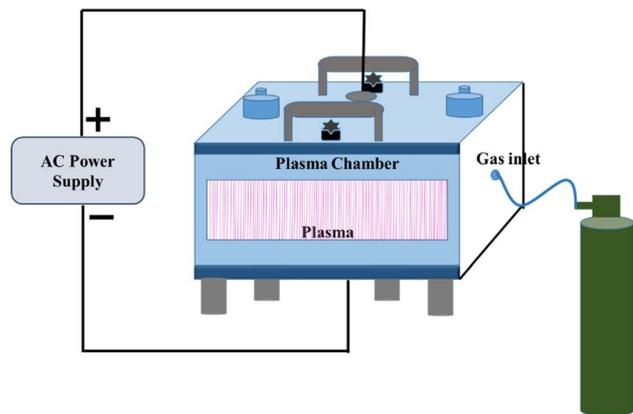
Fig. 1 Schematic representation of DBD plasma system.
