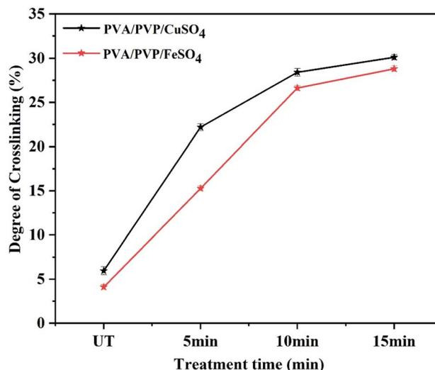
Fig. 9 Degree of crosslinking of PVA/PVP/CuSO<sub>4</sub> and PVA/PVP/FeSO<sub>4</sub> polymer films.
