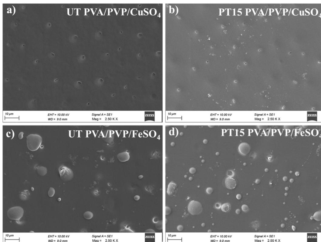
Fig. 7 SEM analysis of PVA/PVP/CuSO<sub>4</sub> and PVA/PVP/FeSO<sub>4</sub> polymer films.
