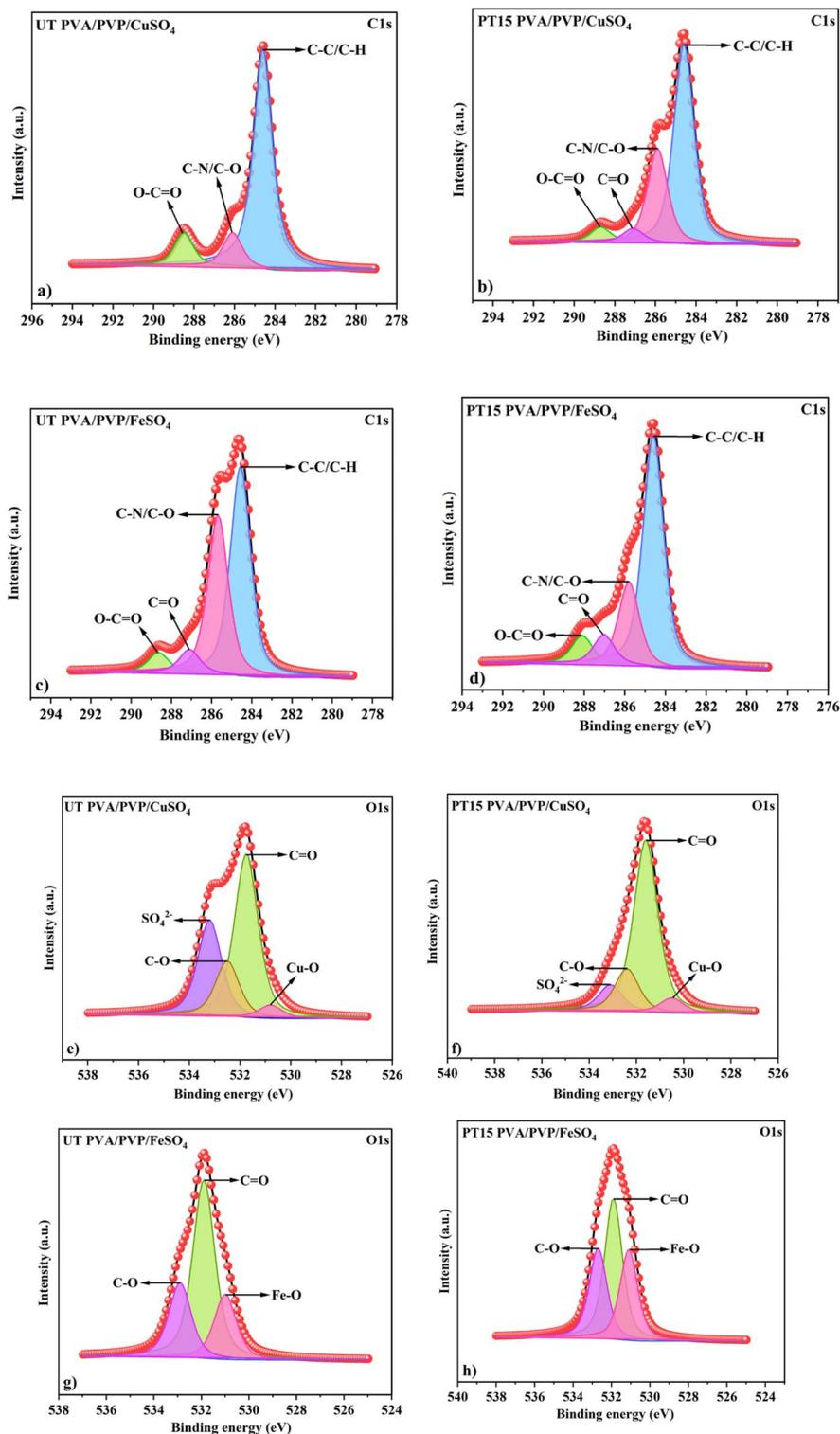
Fig. 6 Deconvoluted peaks of (a) C1s UT PVA/PVP/CuSO<sub>4</sub> (b) C1s PT15 PVA/PVP/CuSO<sub>4</sub> (c) C1s UT PVA/PVP/FeSO<sub>4</sub> (d) C1s PT15 PVA/PVP/FeSO<sub>4</sub> (e) O1s UT PVA/PVP/CuSO<sub>4</sub> (f) O1s PT15 PVA/PVP/CuSO<sub>4</sub> (g) O1s UT PVA/PVP/FeSO<sub>4</sub> (h) O1s PT15 PVA/PVP/FeSO<sub>4</sub>.
