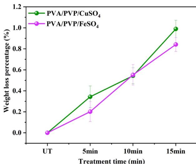
Fig. 2 Weight loss analysis of polymer films after plasma treatment.
