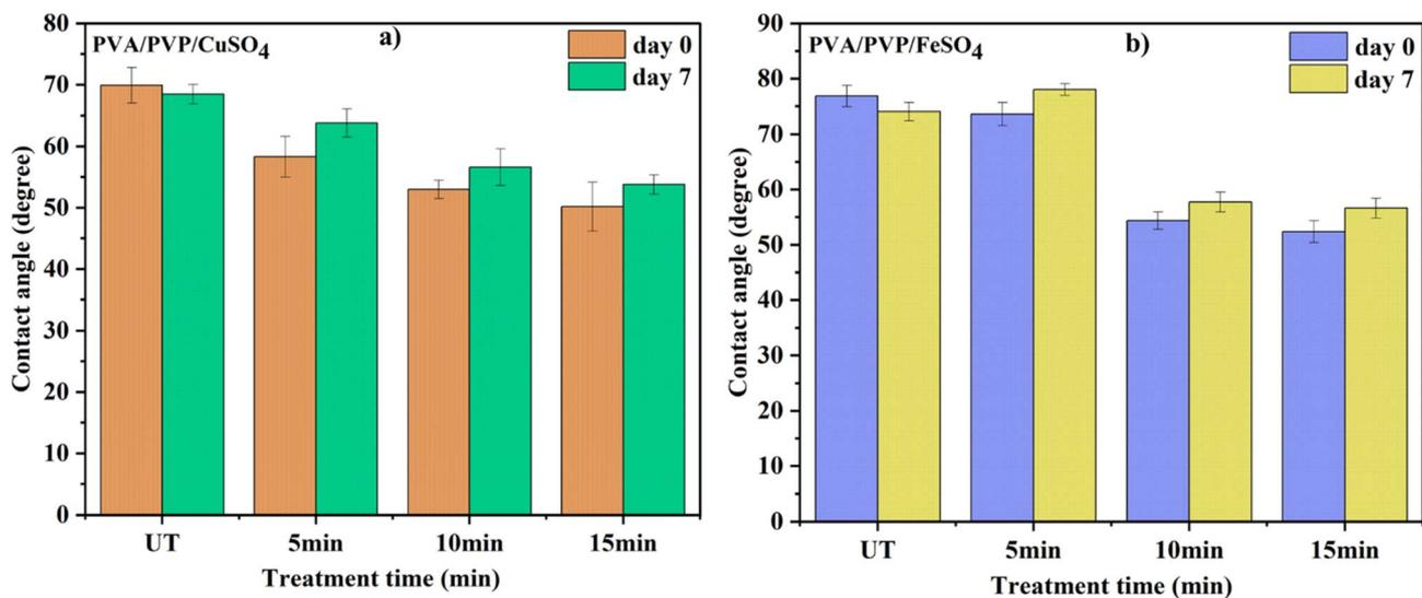
Fig. 4 Aging analysis of (a) PVA/PVP/CuSO<sub>4</sub> and (b) PVA/PVP/FeSO<sub>4</sub> polymer films.
