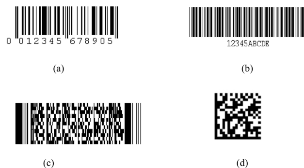
Fig. 3 Different types of barcodes: (a) EAN-13, (b) Code 39, (c) PDF-417, and (d) data matrix code. Reprinted (adapted) with permission from ref. 44. Copyright © 2006 Elsevier Ltd.
