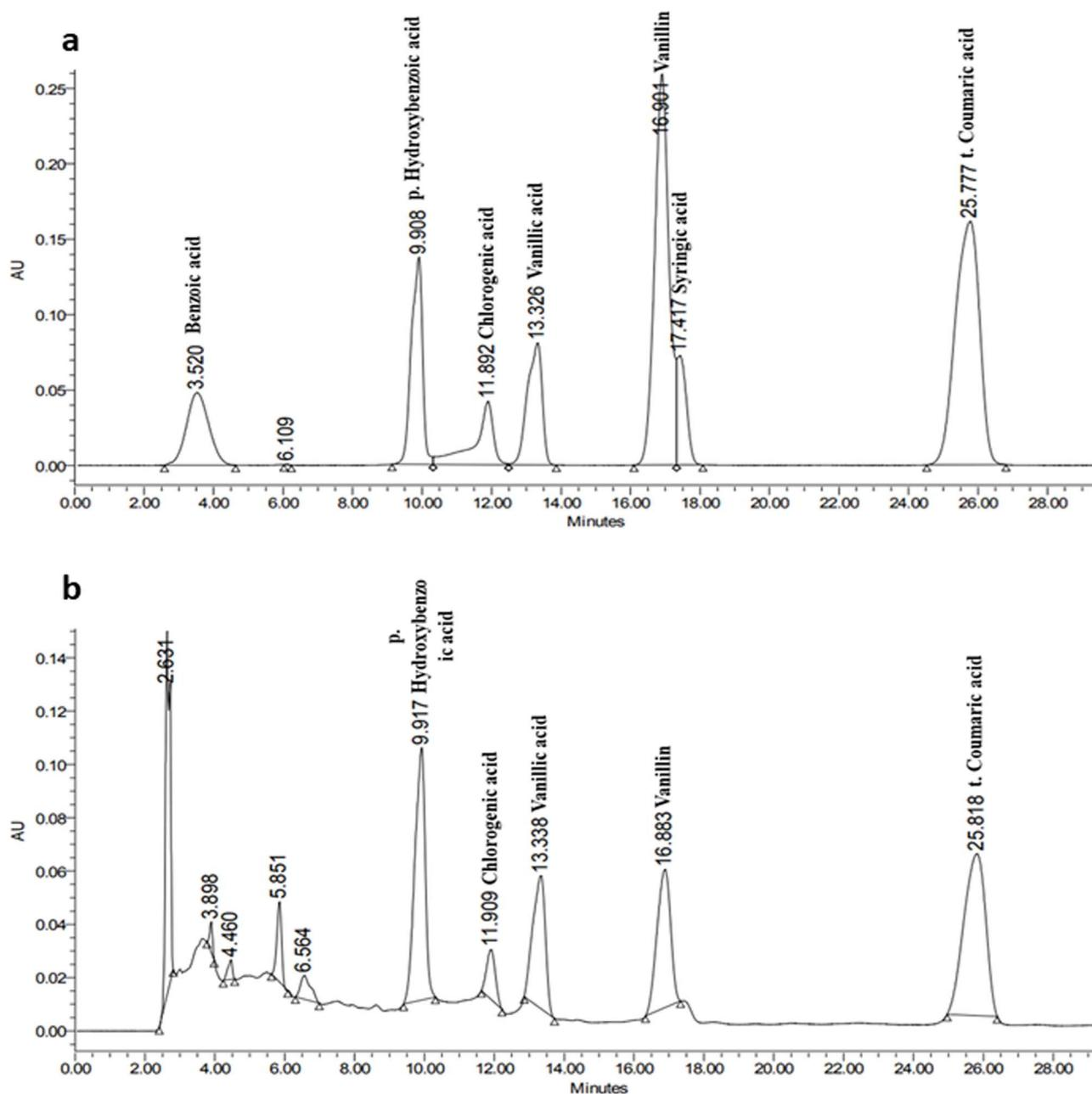
Fig. 5 (a) UPLC-chromatogram of phenolic standards: benzoic acid, hydroxybenzoic acid, chlorogenic acid, vanillic acid, vanillin, syringic acid, and *p*-coumaric acid. (b) Determination of phenolic compounds in SFE-LS optimized extract.
