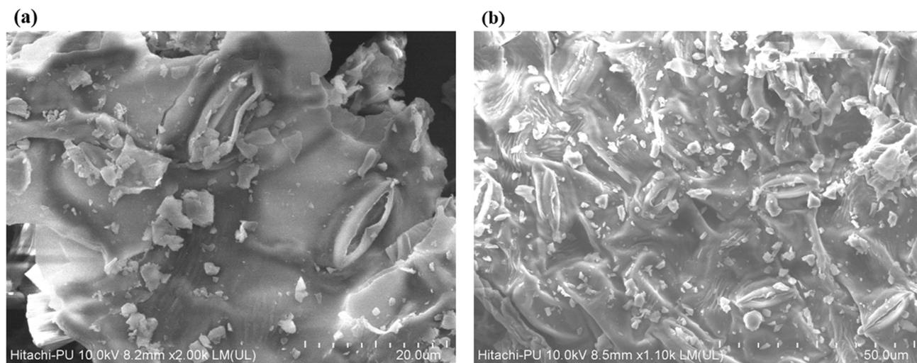
**Fig. 4** FESEM image of LS powder: (a) before extraction and (b) after extraction.
