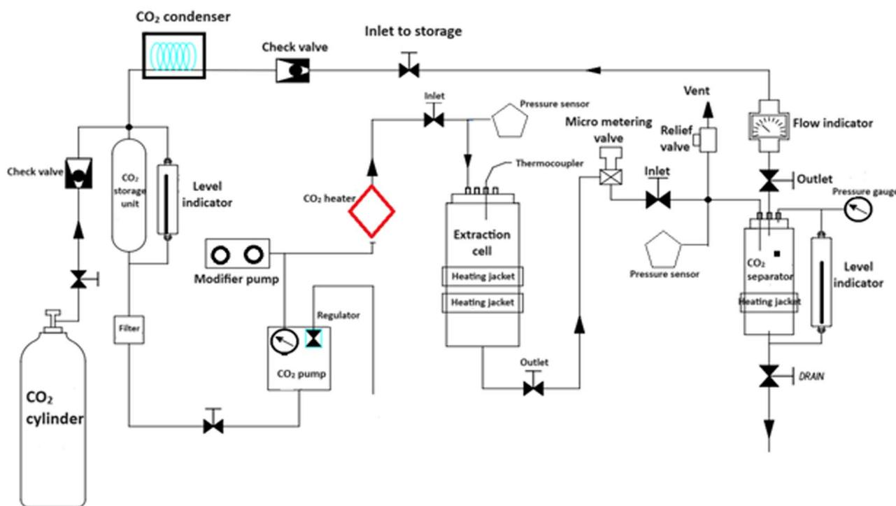
Fig. 1 The process flow of supercritical CO<sub>2</sub> extraction for total phenolic content (TPC).
