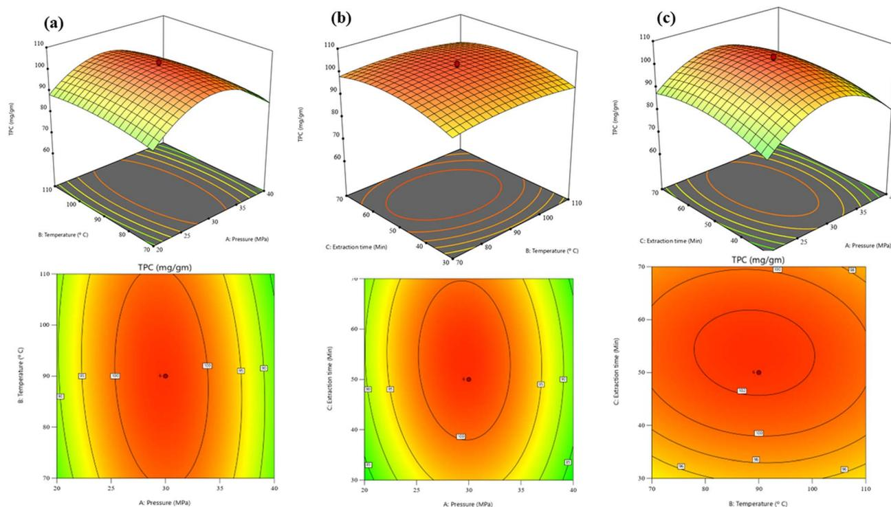
**Fig. 3** The response surface plot shows the effect of two SC-CO<sub>2</sub> parameters on total phenolic content yield (mg per g of DWB): (a) total phenolic content yield vs. extraction temperature and pressure with a constant extraction time of 50 min, (b) total phenolic content yield vs. extraction time and temperature with a constant pressure of 30 MPa, and (c) total phenolic content yield vs. extraction time and pressure with a constant temperature of 90 °C.
