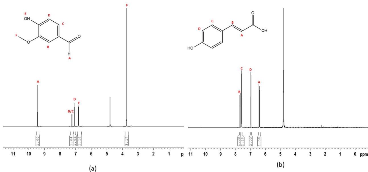
Fig. 7 (a) ^1\text{H} NMR for fraction 29 (vanillin) and (b) ^1\text{H} NMR for fraction 31 ( p -coumaric acid).
