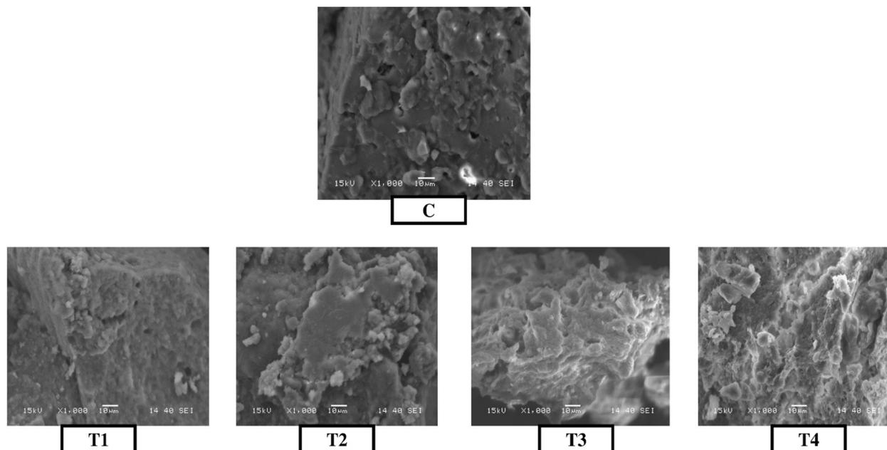
Fig. 4 SEM images of native and cold-plasma-treated mustard protein isolate.
