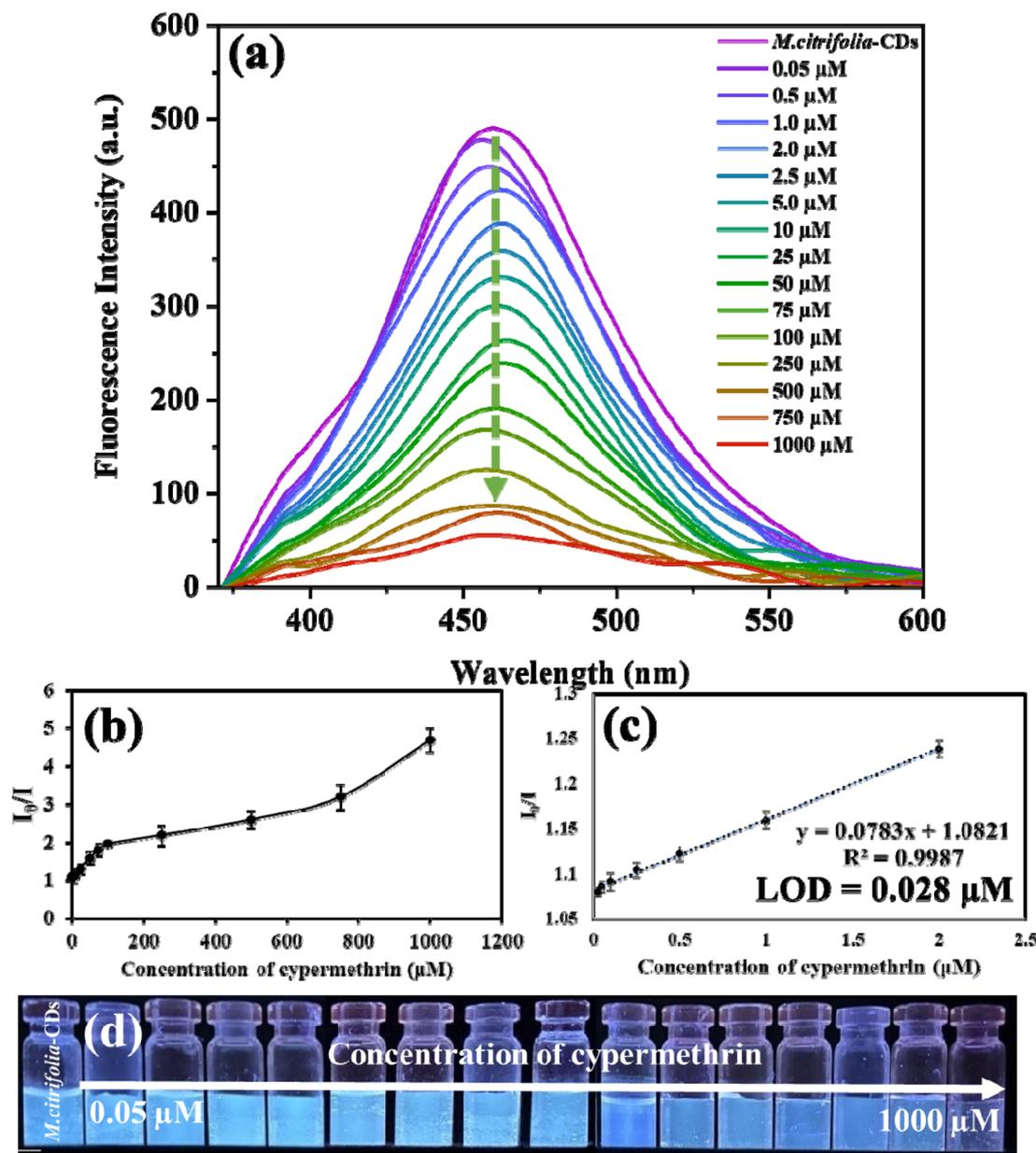
Fig. 7 (a) Fluorescence emission spectra of *M. citrifolia*-CDs after addition of different concentrations of cypermethrin (0.05–1000  $\mu\text{M}$ ) solutions. (b) Stern–Volmer plot between  $I_0/I$  and concentrations of cypermethrin. (c) Calibration curve plotted between  $I_0/I$  and concentrations of cypermethrin. (d) The photographic representation of fluorescence changes in *M. citrifolia*-CDs with an increasing concentration of cypermethrin under a UV lamp at 365 nm.
