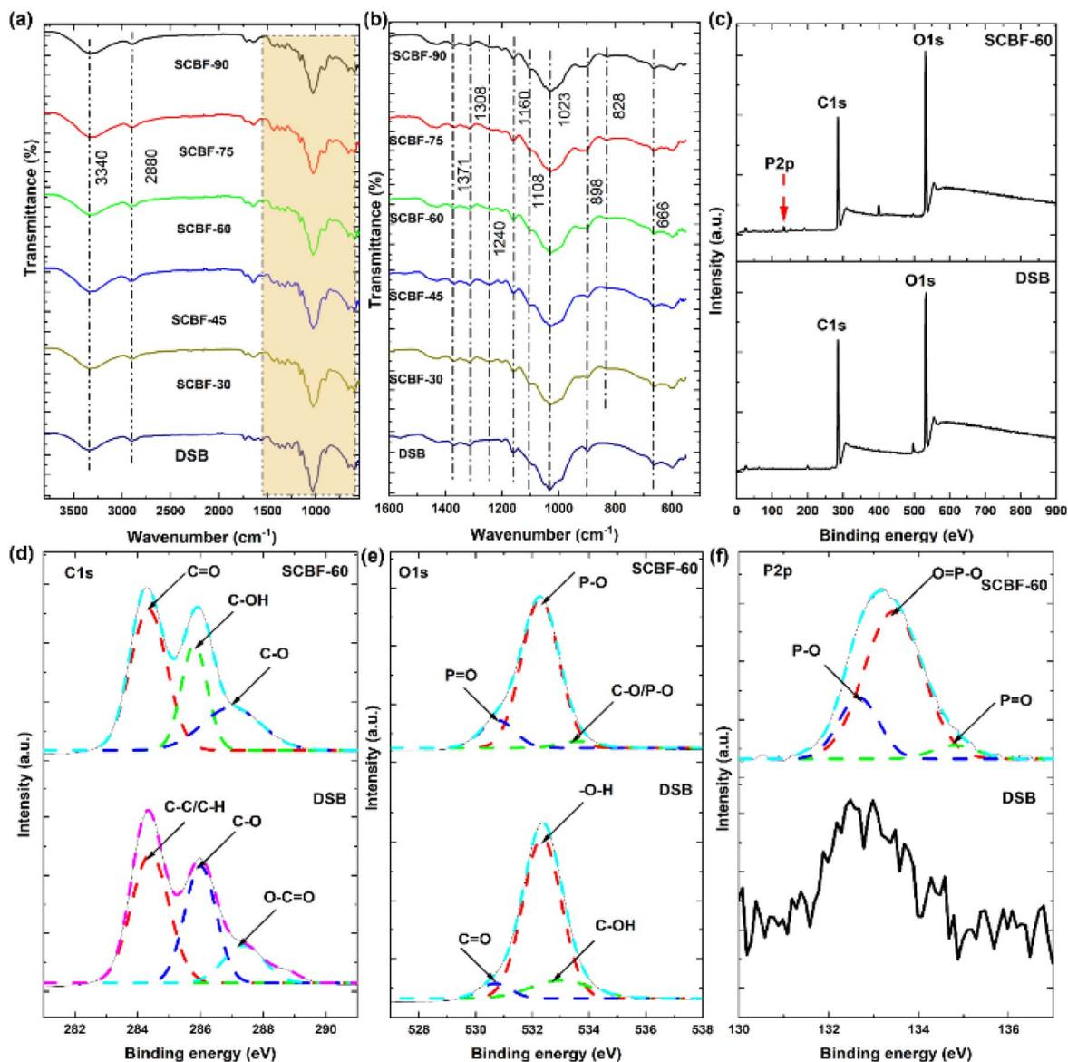
Fig. 2 FTIR spectra of SCBF films in the range of (a) 600–4000  $\text{cm}^{-1}$  and (b) 600–1600  $\text{cm}^{-1}$ . (c) XPS survey of DSB and SCBF-60, (d) C1s, (e) O1s, and (f) P2p bonds of DSB and SCBF-60.
