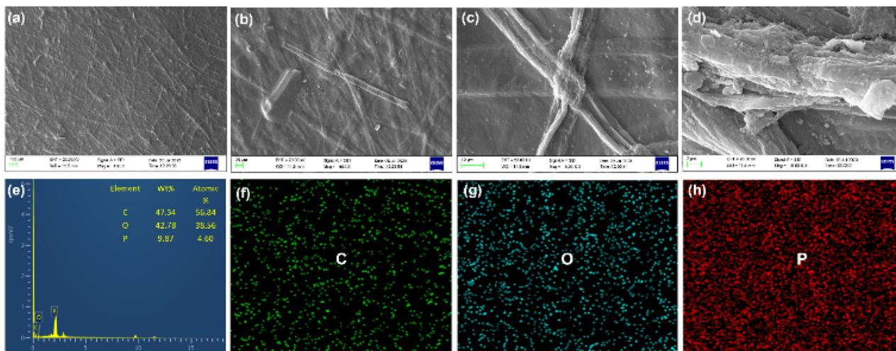
Fig. 3 SEM micrograph of SCBF films, (a) 100 $\times$ , (b) 500 $\times$ , (c) 3k $\times$ , and (d) 10k $\times$ , (e) EDS analysis with elemental mapping of (f) carbon, (g) oxygen, and (h) phosphorus, respectively.
