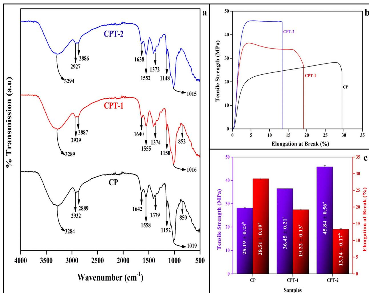
Fig. 1 (a) FTIR analysis, mechanical properties (b) stress vs. strain curve and (c) TS and EB of control CP and CPT intelligent biodegradable films.
