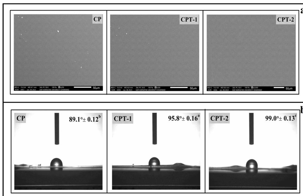
Fig. 2 (a) SEM micrographs and (b) water contact images of control CP and CPT intelligent biodegradable films.
