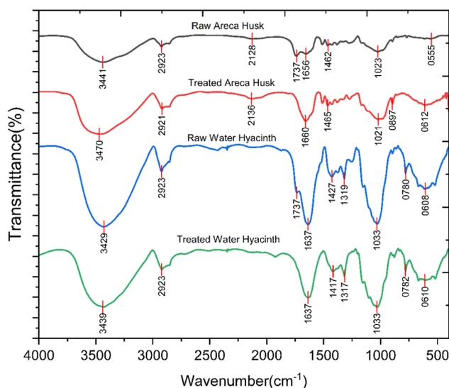
Fig. 1 FTIR spectra of raw and alkali-treated fibers.
