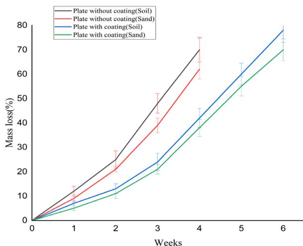
Fig. 6 Biodegradability analysis of coated and non-coated plates.
