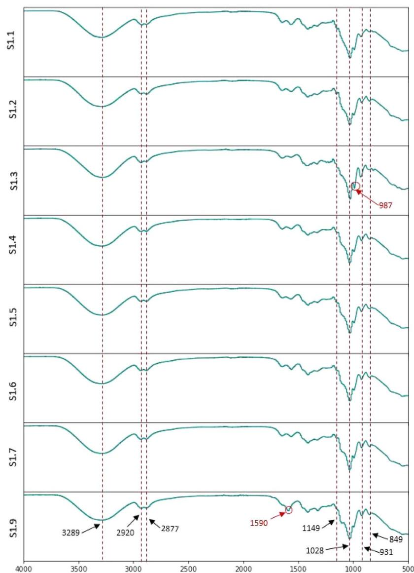
Fig. 1 FTIR spectroscopy of the film samples.
