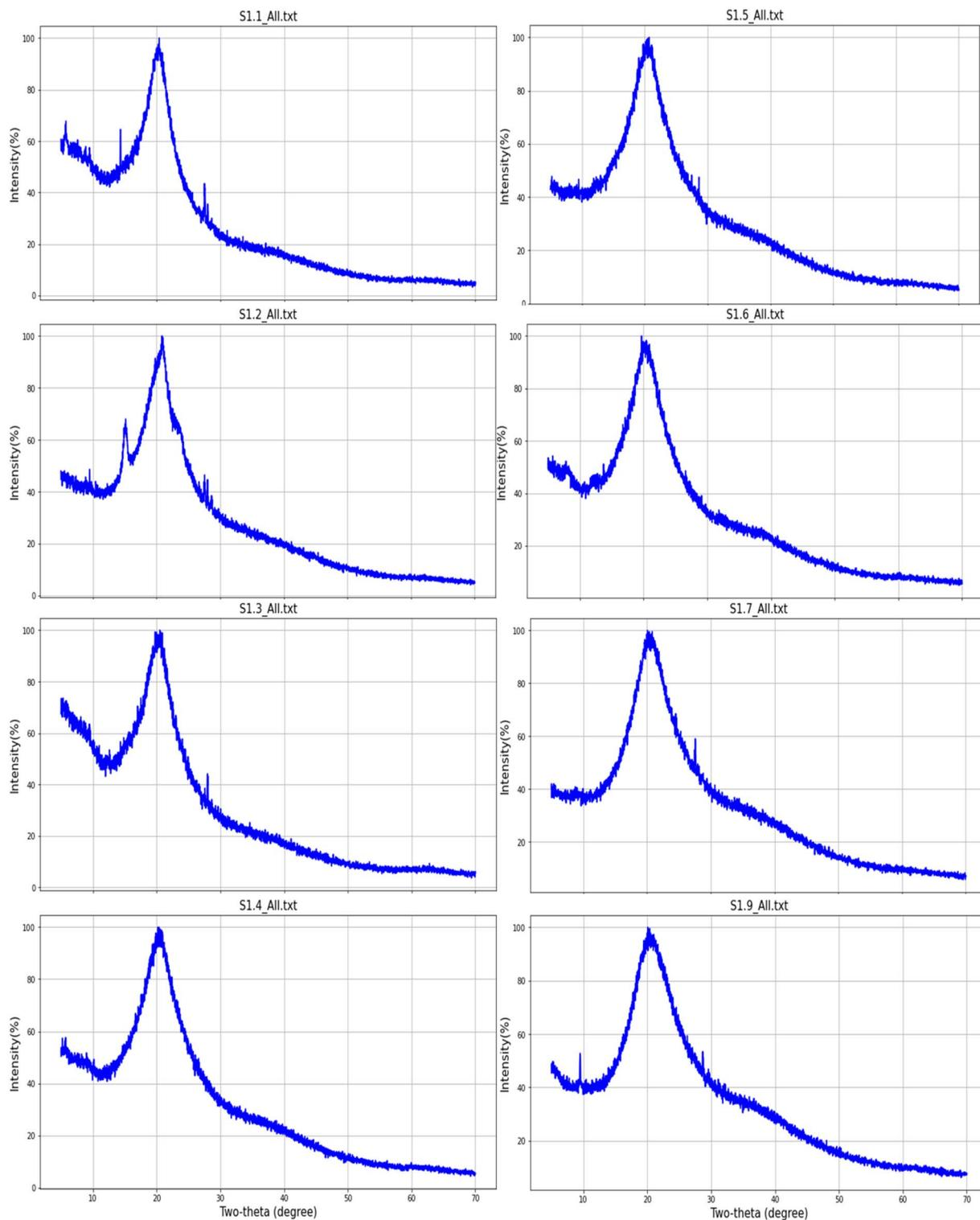
Fig. 2 XRD of film samples.
