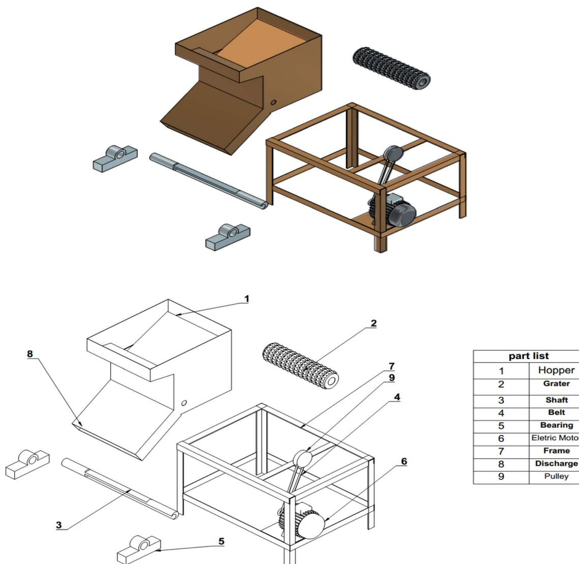
Fig. 1 An assembly drawing of the cassava grater and an exploded view showing all components of the cassava grater system.
