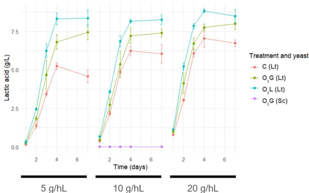
Fig. 3 Evolution of lactic acid concentration ( $\text{g L}^{-1}$ ) during fermentation. The figure shows the average obtained for the different treatments (C, O<sub>3</sub>G and O<sub>3</sub>L) grouped according to the concentration of the added inoculum of *L. thermotolerans* (Lt) or *S. cerevisiae* (Sc) (5, 10 and 20  $\text{g hL}^{-1}$ ). The error bars correspond to the standard deviation associated with each average.
