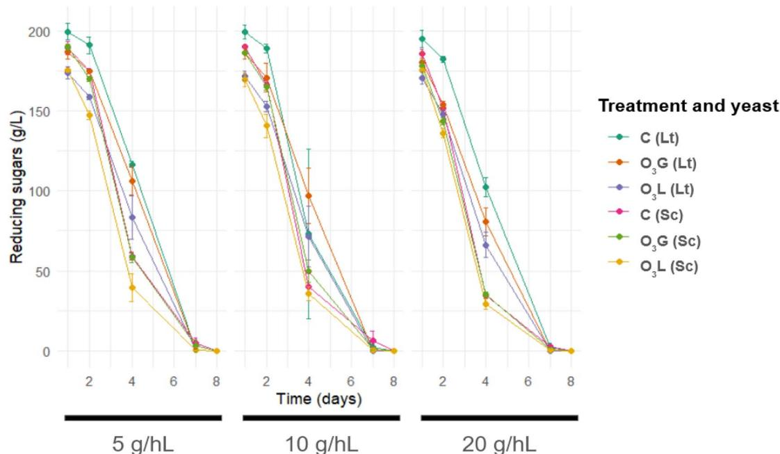
Fig. 2 Evolution of reducing sugar concentration ( $\text{g L}^{-1}$ ) during fermentation. The figure shows the mean obtained for the different treatments (C, O<sub>3</sub>G and O<sub>3</sub>L) grouped according to the concentration of *L. thermotolerans* (Lt) or *S. cerevisiae* (Sc) inoculum added (5, 10 and 20  $\text{g hL}^{-1}$ ). Error bars represent the standard deviation associated with each mean.
