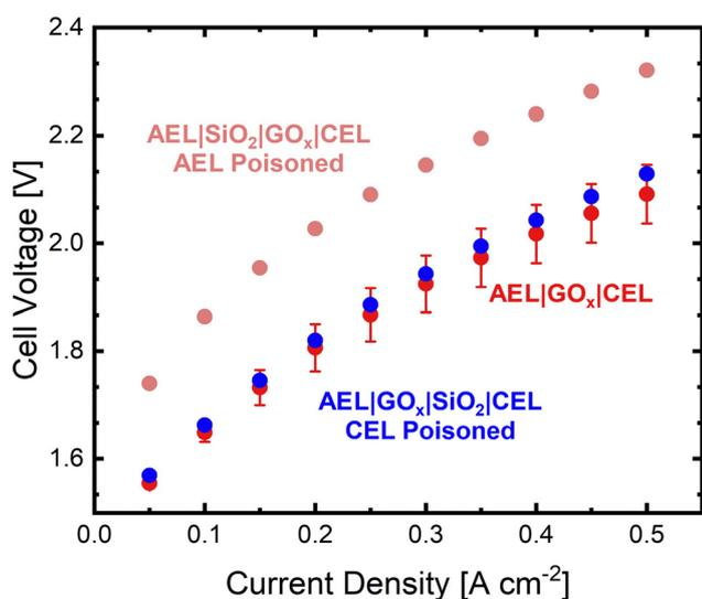
Fig. 5 Polarization curves of GO<sub>x</sub> BPMs poisoned with SiO<sub>2</sub> on either the CEL or AEL. SiO<sub>2</sub> sprayed onto the AEL substantially reduces performance, whereas SiO<sub>2</sub> sprayed onto CEL only minimally impacts performance.
