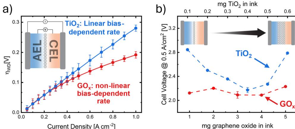
Fig. 2 Current–voltage response and loading dependence of  $TiO_2$  and  $GO_x$  BPMs. (a) Full-cell potential vs. current density of the BPM water electrolyzers. (b) Dependence of WD-catalyst loading on polarization response. All measurements recorded at  $55^\circ C$ .
