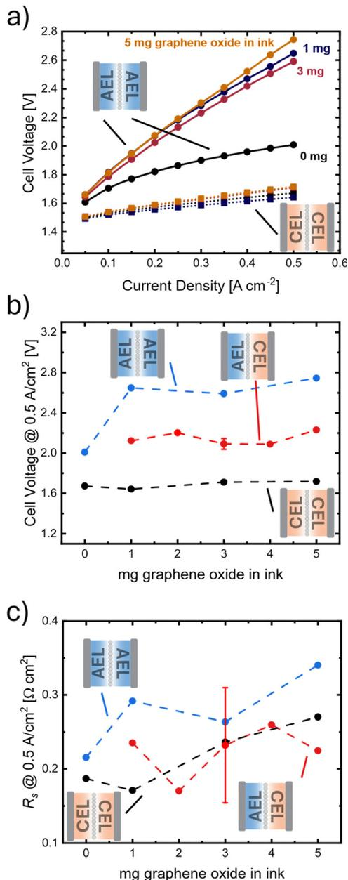
Fig. 3 The impact of  $\text{GO}_x$  WD catalysts loading in BPMs (a) *i*-*V* curves for the AEL| $\text{GO}_x$ |AEL and CEL| $\text{GO}_x$ |CEL devices with various  $\text{GO}_x$  loadings. (b) The cell voltage of CEL, AEL, and BPM devices as a function of the interlayer  $\text{GO}_x$  loading. (c) The high-frequency resistance increases only slightly as a function of  $\text{GO}_x$  loading for all architectures.
