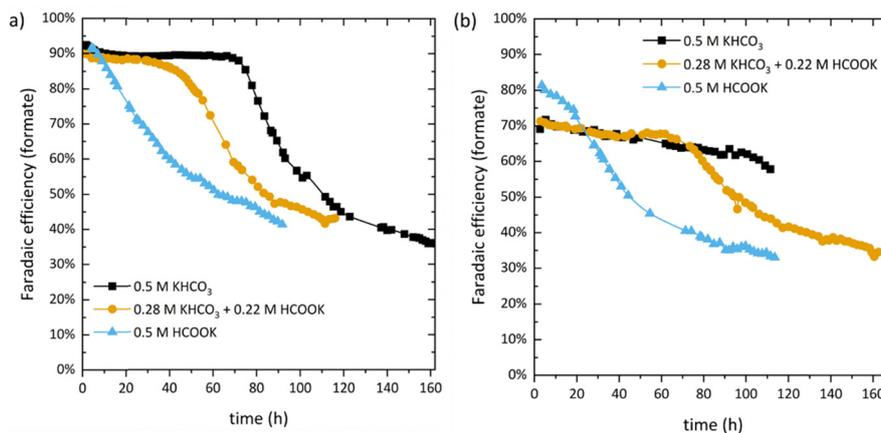
Fig. 4 Time dependent evolution of the FE ( $\text{HCOO}^-/\text{HCOOH}$ ) in a series of long-term control experiments with a current density of  $100 \text{ mA cm}^{-2}$  and changing the catholyte composition while using (a) Bi GDE; and (b) Sn GDE as cathode.
