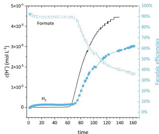
Fig. 5 Time dependence of proton concentration in the catholyte (left y-axis) and faradaic efficiencies towards formate and  $\text{H}_2$  (right y-axis) in an ECR experiment in 0.5 M  $\text{KHCO}_3$  catholyte solution and  $100 \text{ mA cm}^{-2}$ .
