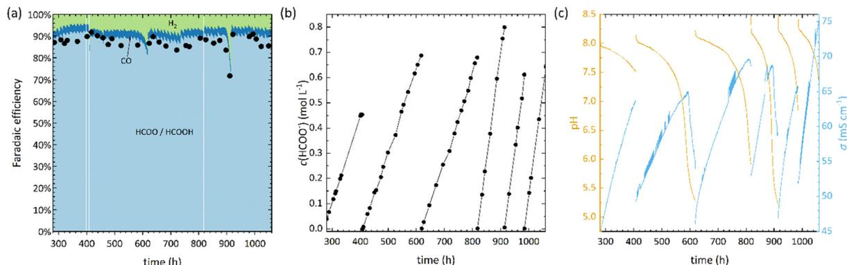
Fig. 6 Reactivation Zone: continuous operation from 275–1075 hours of Bi GDE at  $100 \text{ mA cm}^{-2}$ , with evolution over time of (a) faradaic efficiency of products, (b) formate concentration in the catholyte reservoir, and (c) pH (left) and conductivity (right) of the catholyte. Data shown are from the same continuous experiment.
