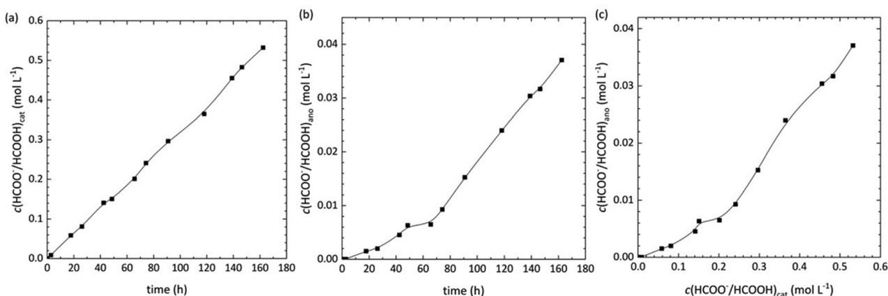
Fig. 3 Time-dependent formate concentrations in the (a) catholyte and (b) anolyte during long-term electrolysis with Bi GDE at  $100 \text{ mA cm}^{-2}$ , demonstrating crossover through the bipolar membrane contributing to differences between GC- and HPLC-derived faradaic efficiencies (cf. Fig. 2a). (c) The FA concentration in the anolyte is plotted against that in the catholyte. Data shown are from the same continuous experiment.
