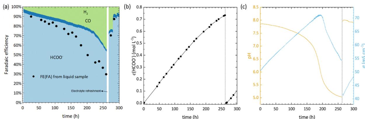
Fig. 2 The initial 300 hours of Bi GDE at  $100 \text{ mA cm}^{-2}$ , depicting the stability and degradation zones, during which process the change of (a) faradaic efficiency of products, (b)  $HCOO^-$  concentration in the catholyte, and (c) pH (left y-axis) and conductivity (right y-axis) of the catholyte are plotted against time. Data shown are from the same continuous experiment.
