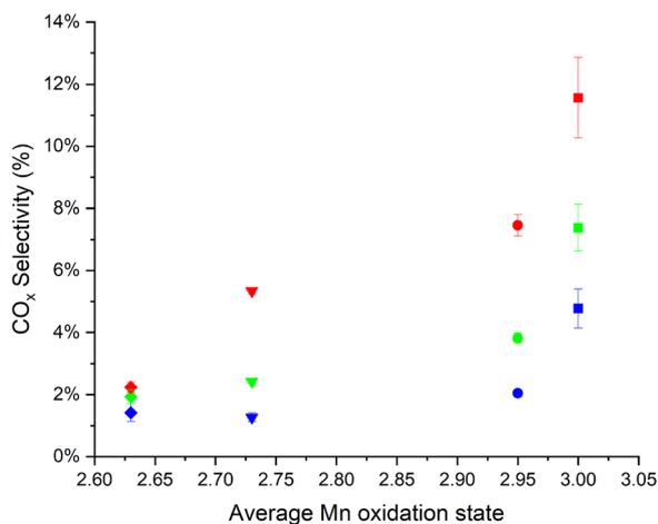
**Fig. 9** CO<sub>x</sub> selectivity vs. computed average starting Mn oxidation state for 4% O<sub>2</sub> reoxidation (diamond), 10% O<sub>2</sub> reoxidation (triangle), 20 min post oxidation purge, and (square) 5 min. post oxidation purge at (blue) 800 °C, (green) 825 °C, and (red) 850 °C. Note that a few error bars are too small to be clearly visible.
