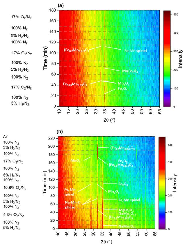
Fig. 6 *In situ* XRD of (a) NaW-( $\text{Fe}_{0.1}\text{Mn}_{0.9}$ ) $_x\text{O}_y$  and (b) NaMgW-( $\text{Fe}_{0.1}\text{Mn}_{0.9}$ ) $_x\text{O}_y$  subjected to 5%  $\text{H}_2$  redox cycles at 850 °C. FeO and MnO phases form during reduction but the intensity is too low to be distinguishable on this scale.
