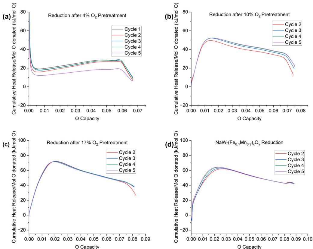
Fig. 8 Average heat release/mol O donated for (a) NaMgW–(Fe<sub>0.1</sub>Mn<sub>0.9</sub>)<sub>x</sub>O<sub>y</sub> cycled with 4% O<sub>2</sub>, (b) cycled with 10% O<sub>2</sub>, (c) cycled with 17% O<sub>2</sub>, and (d) NaW–(Fe<sub>0.1</sub>Mn<sub>0.9</sub>)<sub>x</sub>O<sub>y</sub> cycled with 17% O<sub>2</sub>.
