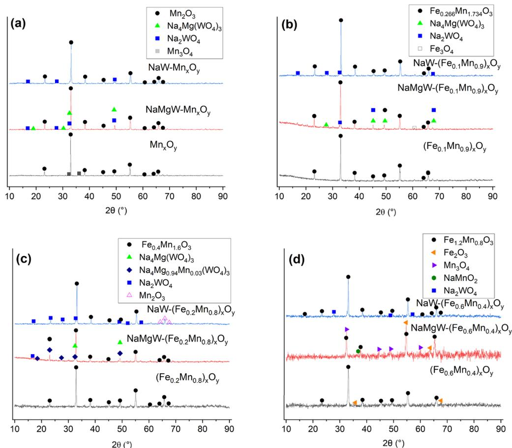
Fig. 2 Ex situ XRD of synthesized (a)  $\text{Mn}_x\text{O}_y$ , (b)  $(\text{Fe}_{0.1}\text{Mn}_{0.9})_x\text{O}_y$ , (c)  $(\text{Fe}_{0.2}\text{Mn}_{0.8})_x\text{O}_y$ , and (d)  $(\text{Fe}_{0.6}\text{Mn}_{0.4})_x\text{O}_y$  catalysts.
