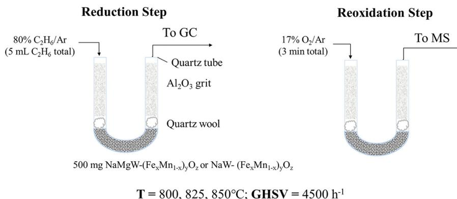
Fig. 1 Schematic for CL-ODH catalyst activity testing.
