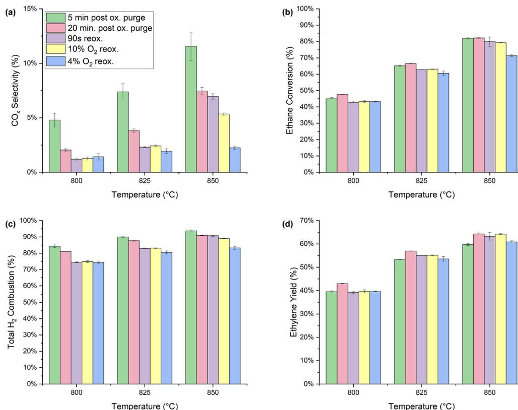
Fig. 5 (a) CO<sub>x</sub> selectivity, (b) ethane conversion, (c) total H<sub>2</sub> combustion, and (d) ethylene yield results from NaMgW-(Fe<sub>0.1</sub>Mn<sub>0.9</sub>)<sub>x</sub>O<sub>y</sub> under various oxidation conditions: (green) 5 min. post oxidation purge, (pink) 20 min. post oxidation purge, (purple) 90s reoxidation, (yellow) 10% O<sub>2</sub>/Ar reoxidation, and (blue) 4% O<sub>2</sub>/Ar reoxidation.
