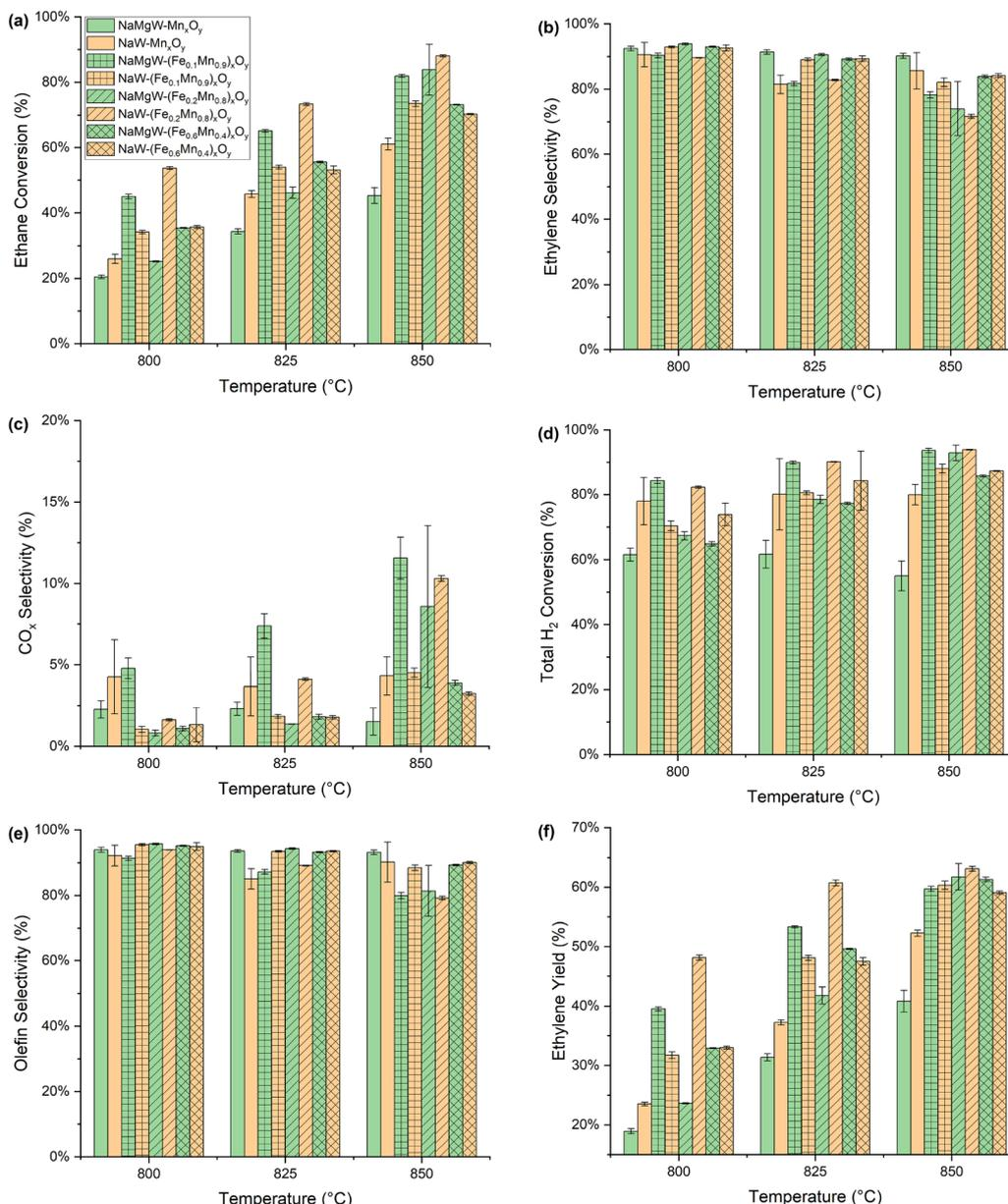
Fig. 3 (a) Ethane conversion, (b) ethylene selectivity, (c)  $\text{CO}_x$  selectivity, (d)  $\text{H}_2$  conversion, (e) total olefin selectivity, and (f) ethylene yield for NaW- and NaMgW-promoted catalysts at 800, 825, and 850 °C with GHSV = 4500  $\text{h}^{-1}$ .
