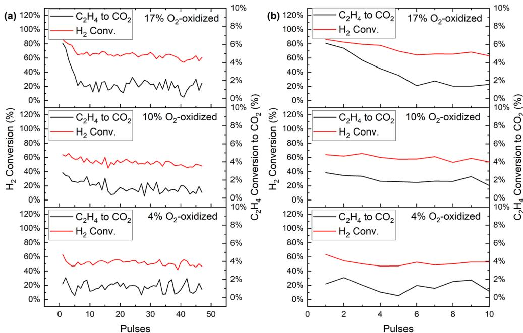
Fig. 7 (a) C<sub>2</sub>H<sub>4</sub> conversion to CO<sub>2</sub> and H<sub>2</sub> conversion over all 50 pulses and (b) over the first 10 pulses with the NaMgW–(Fe<sub>0.1</sub>Mn<sub>0.9</sub>)<sub>x</sub>O<sub>y</sub> catalyst at 850 °C, using 80% C<sub>2</sub>H<sub>4</sub>/20% H<sub>2</sub> 1 mL pulses.
