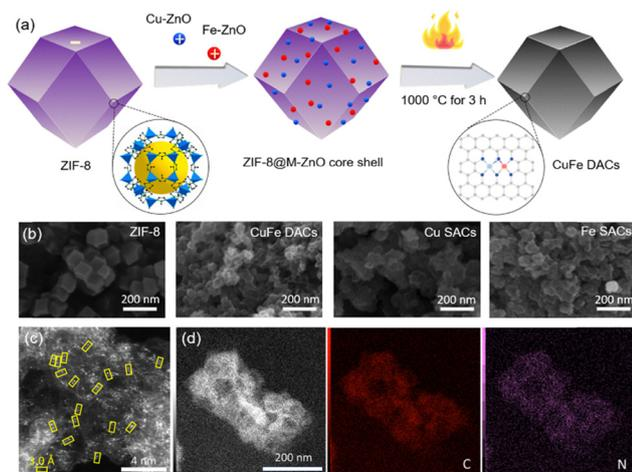
**Fig. 1** (a) The two-step synthetic route of CuFe DACs. (b) SEM images showing the morphological evolution of ZIF-8 to CuFe DACs, Cu SACs, and Fe SACs. (c) AC HAADF-STEM image of CuFe DACs. (d) Corresponding EDS element mapping.
