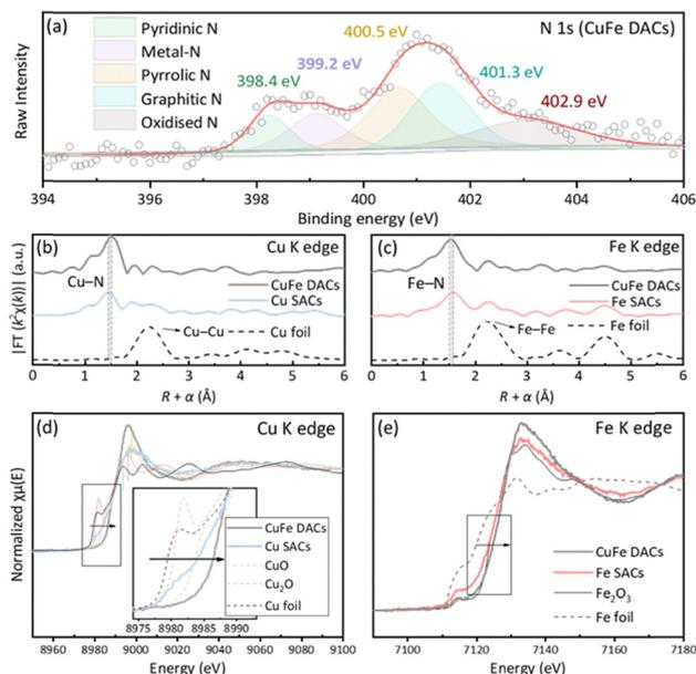
**Fig. 2** (a) N 1s XPS spectrum of CuFe DACs. (b) Cu K-edge FT-EXAFS for CuFe DACs, Cu SACs and Cu foil shown in  $R$ -space. (c) Fe K-edge FT-EXAFS for CuFe DACs, Fe SACs and Fe foil shown in  $R$ -space (the data are  $k^2$ -weighted and not phase-corrected). (d) Cu K-edge XANES for CuFe DACs, Cu SACs, CuO standard, Cu<sub>2</sub>O standard and Cu foil. (e) Fe K-edge XANES for CuFe DACs, Fe SACs, Fe<sub>2</sub>O<sub>3</sub> standard and Fe foil.
