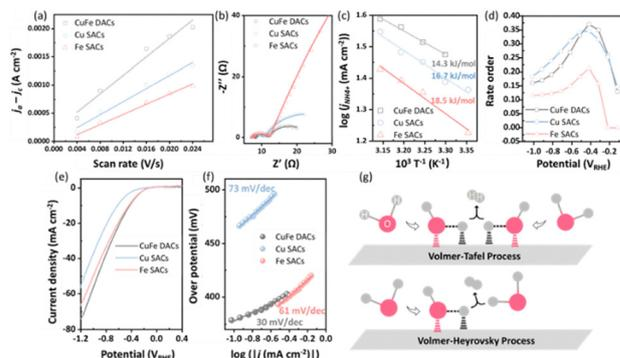
Fig. 4 (a) Capacitive current density as a function of scan rates. (b) EIS spectra. (c) T-dependant  $\text{j}_{\text{NH}_4^+}$ . (d) Potential-dependent reaction rate order. (e) LSV curve in 0.1 M KOH and (f) corresponding Tafel slope for HER on catalysts. (g) Schematic diagram of the Volmer–Tafel (top) and Volmer–Heyrovsky (bottom) processes on a catalyst surface.
