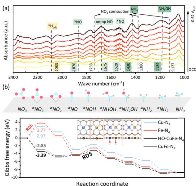
Fig. 5 (a) The *in situ* FTIR spectrum of CuFe DACs in  $\text{NO}_3^-$ -RR via chronoamperometry polarization from open-circuit condition (OCC) to  $-0.62 \text{ V}_{\text{RHE}}$ . (b) Gibbs free energy diagram of various intermediates generated during  $\text{NO}_3^-$ -RR over the  $\text{Cu-N}_4$ ,  $\text{Fe-N}_4$ ,  $\text{HO-CuFe-N}_4$ , and  $\text{CuFe-N}_4$ . Blue, red, and grey balls represent N, O, and H atoms, respectively.
