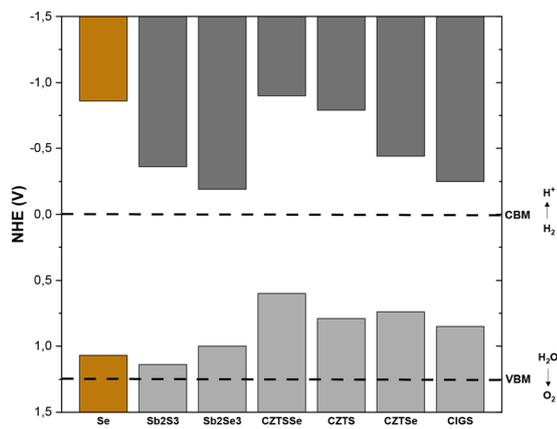
Fig. 4 Band edge positions<sup>28,33,35,37,38,40</sup> of commonly studied photocathode materials relative to NHE, along with the redox potentials required for water splitting.
