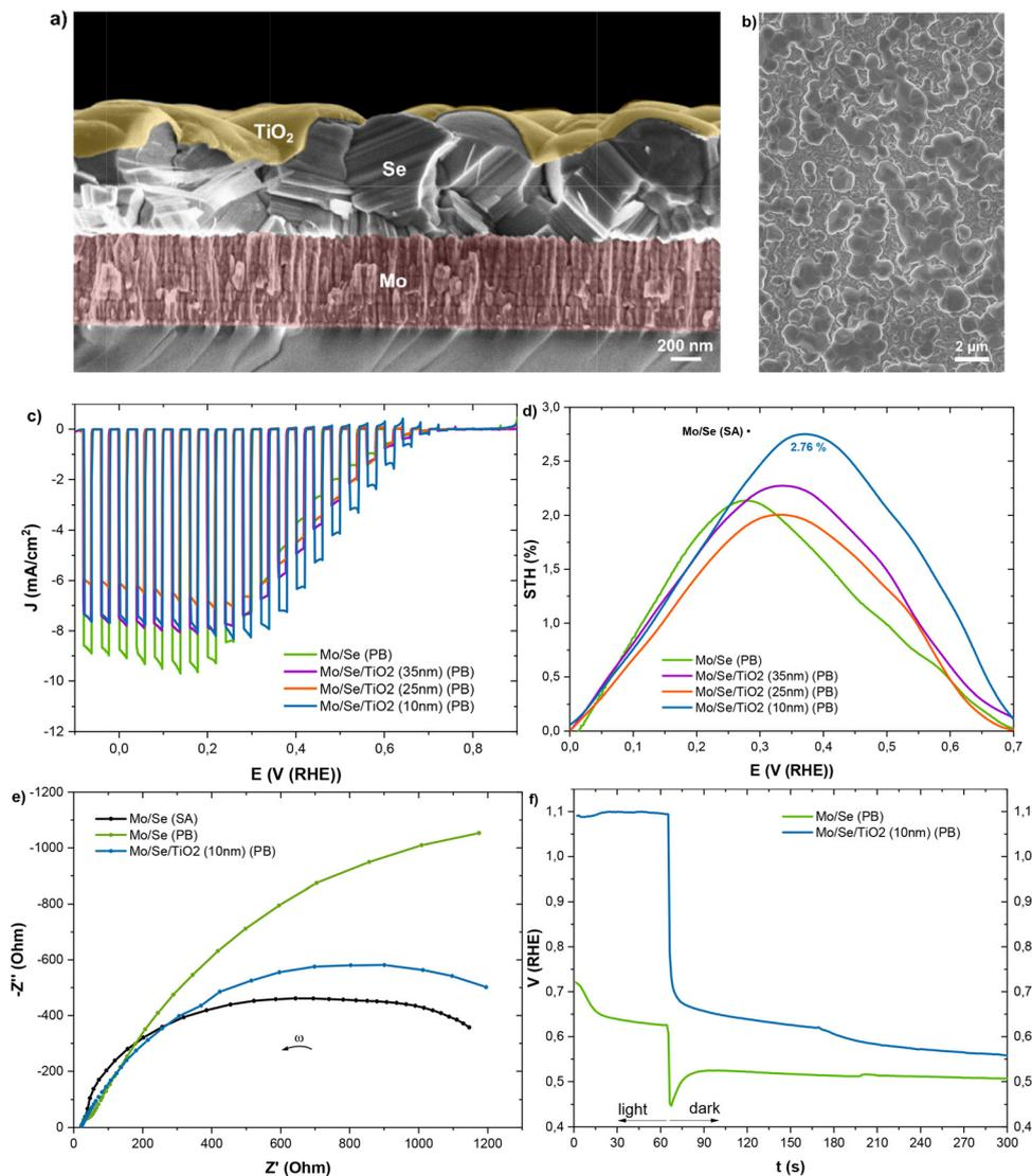
Fig. 2 Cross-sectional SEM image of Mo/Se/TiO<sub>2</sub> (a). Top-view SEM image of Mo/Se (b). *J* under chopped illumination (c) and corresponding HC-STH efficiency (d). Nyquist plots (e). *V*<sub>ocp</sub> measurements (f).
