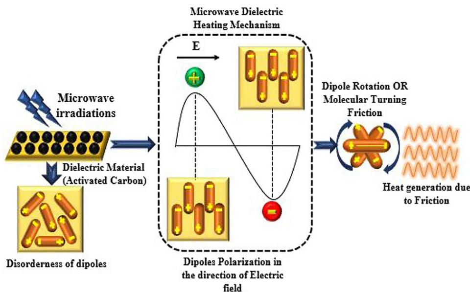
Fig. 4 Dipole polarisation and dipole rotation mechanisms of MW heating on AC as a MW-absorber for polyolefin pyrolysis, reproduced from ref. 48 with permission from Nature Copyright 2023.
