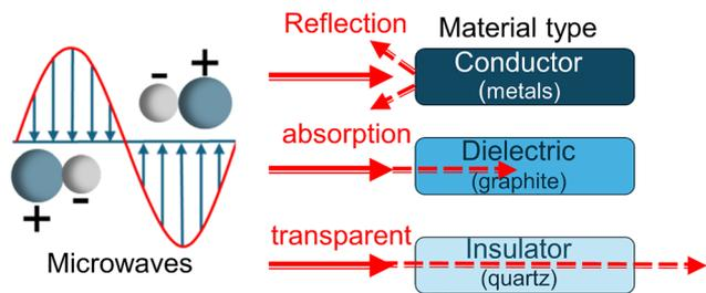
Fig. 2 Classification of solid materials and their interactions with MW conductors, dielectric and insulators, adapted from ref. 38 with permission from MDPI, Copyright 2020.
