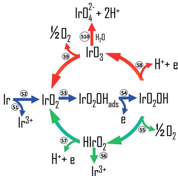
**Fig. 1** Simplified scheme showing possible pathways of Ir dissolution. Green arrows indicate the mechanism that is preferable for electrocatalytically active Ir-based materials at lower potentials. Red arrows present the dissolution route dominating at higher anodic potentials. Blue arrows show intermediate steps that take place regardless of the electrode material and potential. Adapted from ref. 22 with permission from Wiley-VCH, copyrights 2018.
