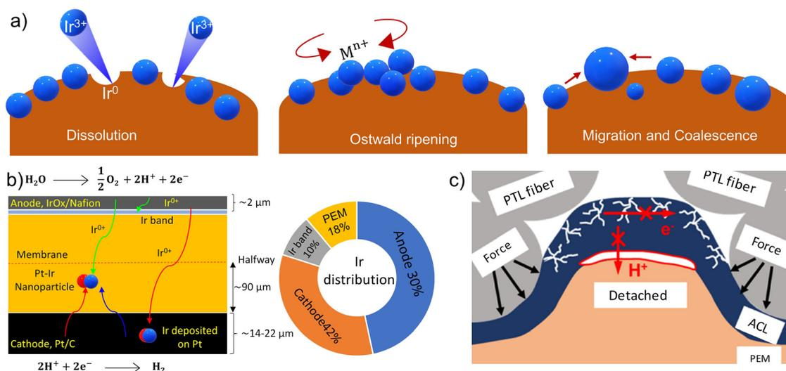
**Fig. 2** (a) Schematic of Ir nanoparticle dissolution, redeposition and coalescence. (b) Diagram depicting the mechanism of Pt–Ir precipitates and Ir band formation in the membrane, with the distribution of Pt and Ir at different regions of the MEA. Adapted from ref. 24 with permission from Elsevier, copyrights 2019. (c) Schematic of the mechanical degradation that takes place in the anode CL. Adapted from ref. 33 with permission from American Chemical Society, copyrights 2024.
