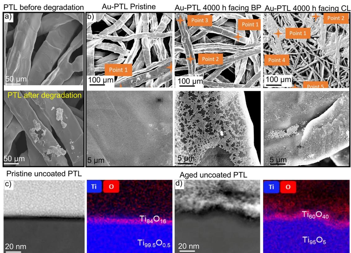
**Fig. 5** PTL degradation and characterizations, (a) SEM images of PTL before and after degradation. Adapted from ref. 72 with permission from Elsevier, copyrights 2018. (b) SEM images of pristine Au-coated PTL; Au-coated PTL that faces the BPP and CL side after 4000 h. (c) High-angle annular dark-field scanning TEM images of pristine uncoated PTL and (d) aged uncoated PTL (left), along with elemental distribution (right). Adapted from ref. 65 with permission from Wiley-VCH, copyrights 2021.
