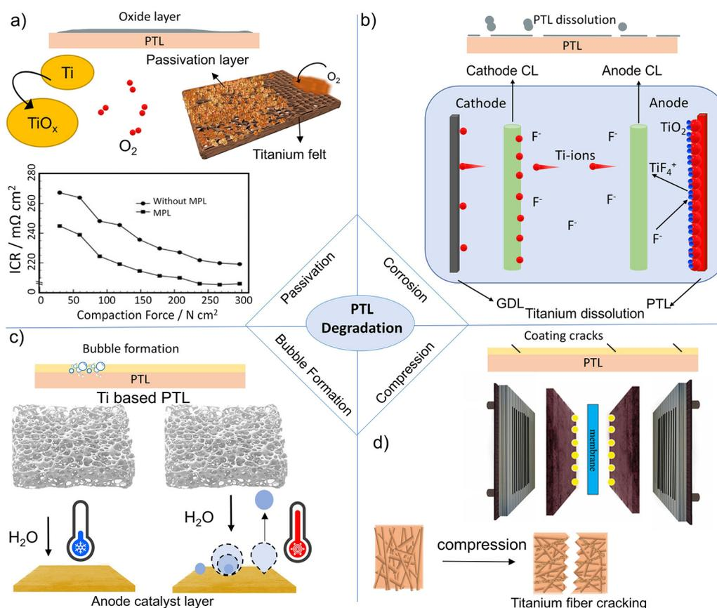
**Fig. 4** Illustration of PTL degradation process in PEMWEs, (a) Schematic illustration of PTL surface passivation. Adapted from ref. 89 with permission from Elsevier, copyrights 2016. (b) Schematic of corrosion mechanism and Ti PTL dissolution. Adapted from ref. 63 with permission from Elsevier, copyrights 2025. (c) Schematic of bubble formation and progression to detachment, (d) Schematic demonstration of mechanical degradation of PTL due to excessive compression force.
