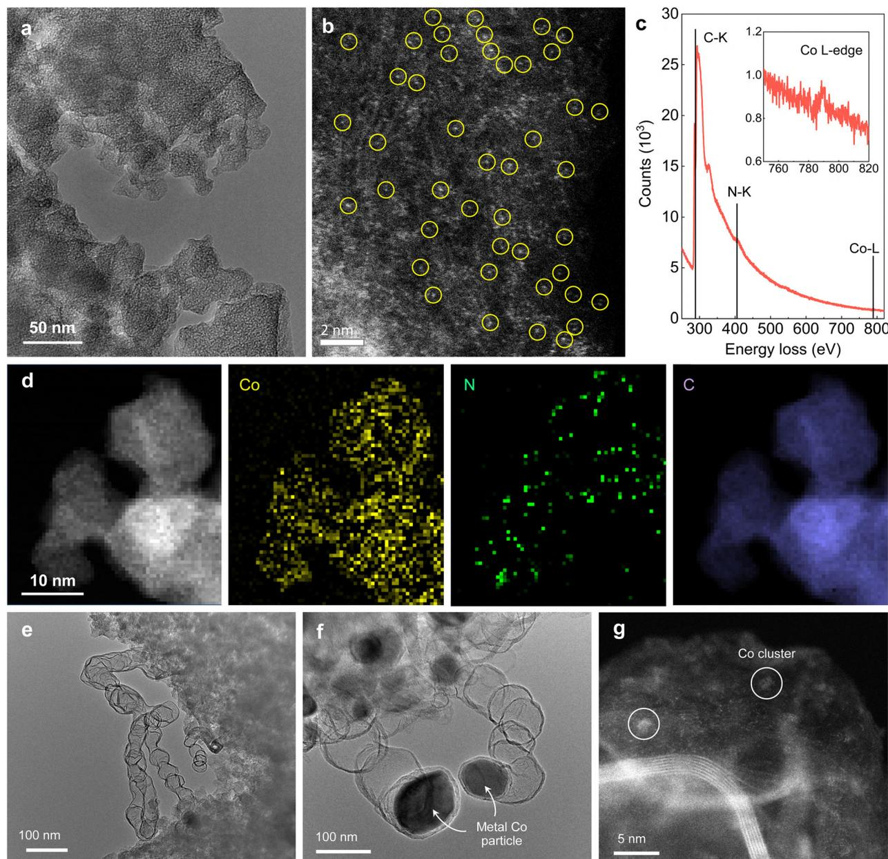
**Fig. 2** Structural characterization of the synthesized Co-N-C catalysts. (a) TEM and (b) HAADF-STEM images of the 3.3Co-NC-1100 catalyst, and Co single atoms highlighted by bright yellow circles in (b). (c) STEM-EELS spectrum of the 3.3Co-NC-1100 catalyst; the inset in (c) showing the enlarged Co L-edge EELS. (d) STEM-EELS elemental mapping of the 3.3Co-NC-1100 catalyst. TEM images of the (e) 5Co-NC-1100 and (f) 10Co-NC-1100 catalysts. (g) HAADF-STEM image of the 5Co-NC-1100 catalyst.
