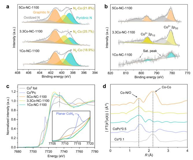
Fig. 3 Spectroscopic characterization of the Co-N-C catalysts. High-resolution (a) N 1s and (b) Co 2p XPS spectra. (c) Co K-edge XANES. (d) Co K-edge Fourier transform of  $k^3$ -weighted EXAFS spectra
