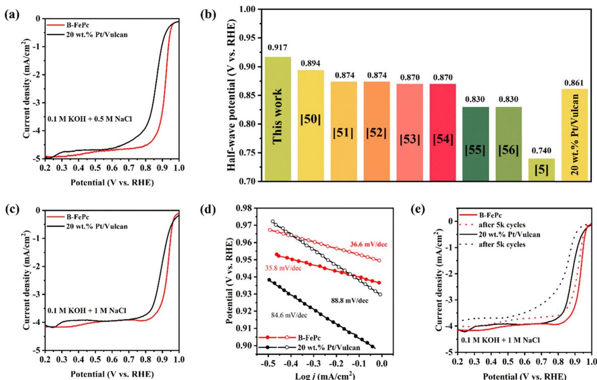
**Fig. 5** (a) Linear sweep voltammetry (LSV) profiles of 20 wt% Pt/C and B-FePc in 0.1 M KOH + 0.5 M NaCl, (b) catalytic activity of recently reported ORR electrocatalysts in alkaline seawater, (c) LSV profiles of 20 wt% Pt/C and B-FePc in 0.1 M KOH + 1 M NaCl, (d) Tafel slopes of 20 wt% Pt/Vulcan and B-FePc calculated from (a, filled) and (c, unfilled) and (e) accelerated stress test results of B-FePc and 20 wt% Pt/Vulcan in 0.1 M KOH + 1 M NaCl after they have undergone 5000 test cycles.
