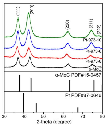
Fig. 6 XRD patterns of the Pt-973-*x* samples.
