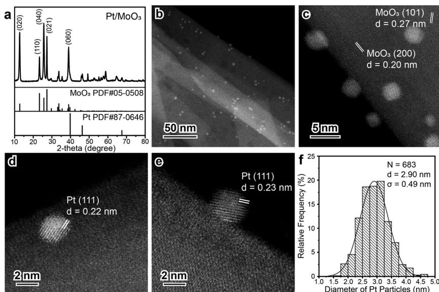
Fig. 1 Structure of the Pt/MoO<sub>3</sub> sample. (a) XRD pattern, (b)–(e) STEM images, and (f) size distribution of Pt particles.
