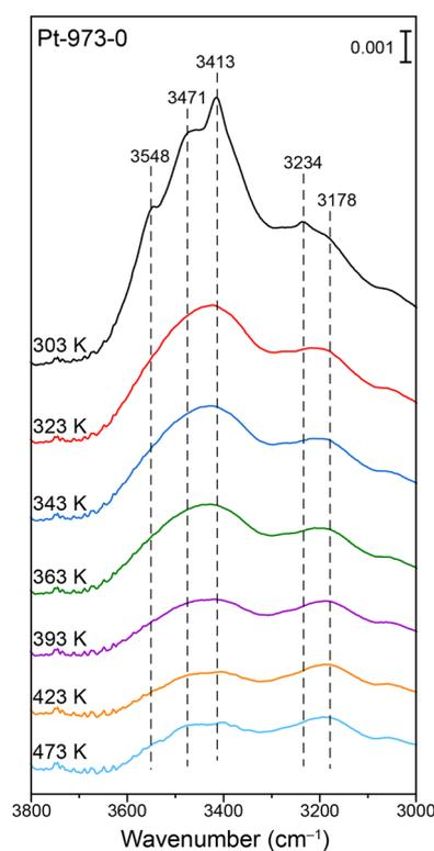
Fig. 11 IR spectra of H<sub>2</sub>O adsorption on the Pt-973-0 catalyst. The spectra were recorded under vacuum ( $1.0 \times 10^{-5}$  mbar) at the specific temperatures.
