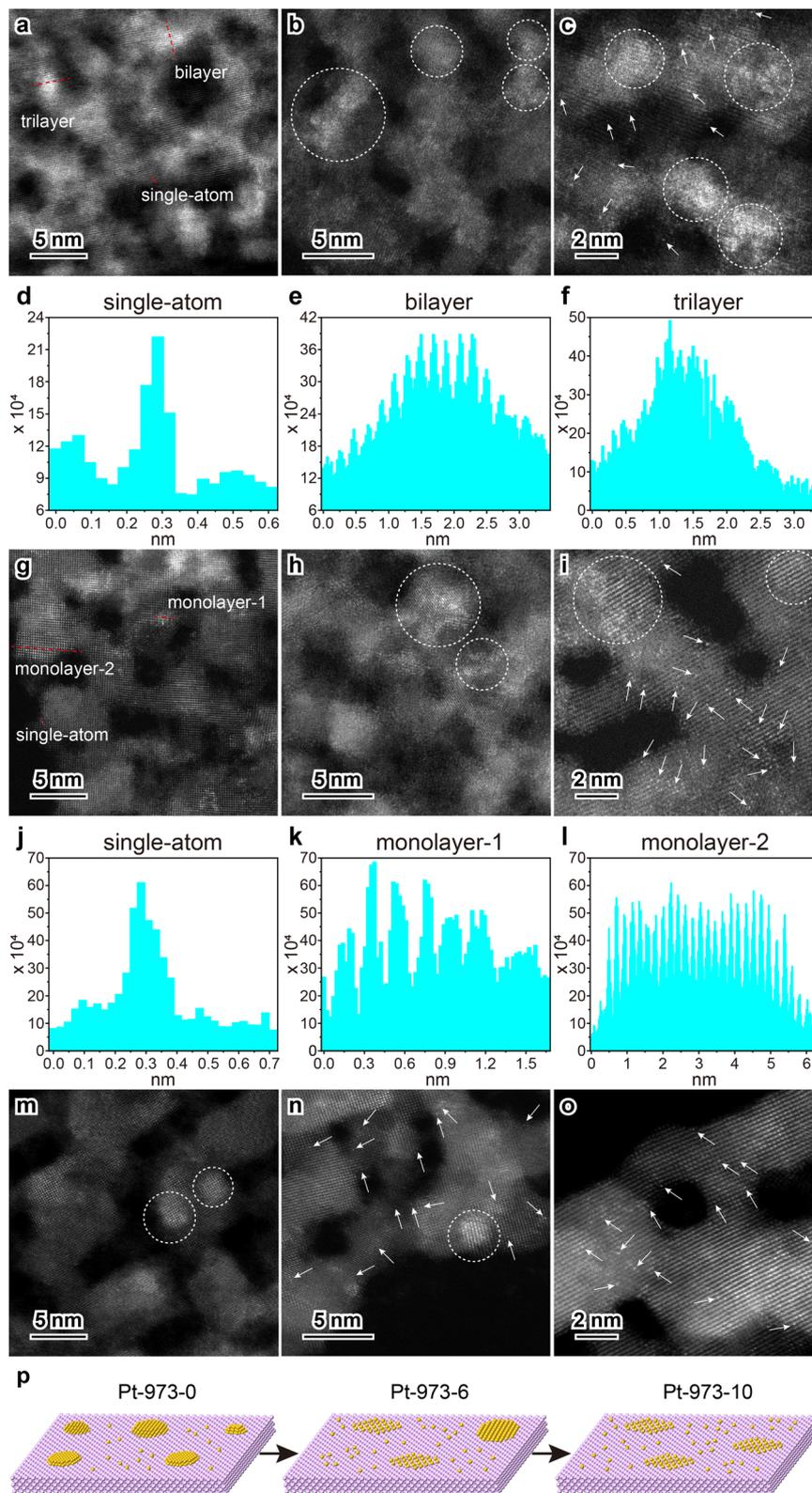
**Fig. 8** Geometric structures of the Pt-973-0 (a)–(f), Pt-973-6 (g)–(l) and Pt-973-10 (m)–(o) samples. Pt thin layers are identified by comparing their line-scanning intensity profiles to those of neighboring Pt single-atoms. (p) A schematic illustration of redistribution of Pt thin layers to single-atoms/monolayers. The circles indicate Pt thin layers, while the arrows indicate Pt single-atoms.
