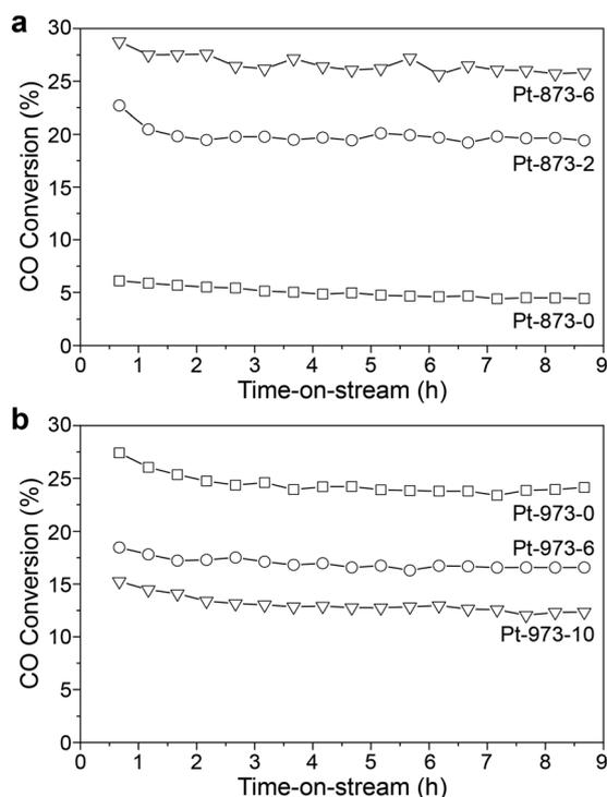
Fig. 10 Low-temperature WGS reaction over the Pt-873-*x* (a) and Pt-973-*x* (b) catalysts. Reaction conditions: 393 K, 3.0 vol% CO/6.0 vol% H<sub>2</sub>O/He, and 50 000 mL g<sup>-1</sup> h<sup>-1</sup>. H<sub>2</sub> and CO<sub>2</sub> are detected as the only products without other by-products under the current reaction conditions.
