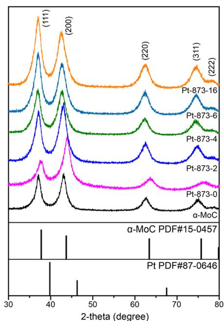
Fig. 2 XRD patterns of the Pt-873-*x* samples.
