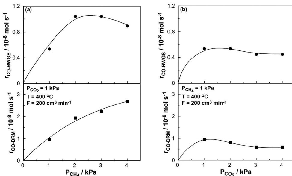
Fig. 4 Steady-state effect of the partial pressure of CH<sub>4</sub> (a) and CO<sub>2</sub> (b) on the catalytic rate of CO production during the DRM (bottom) and RWGS (top) reaction under open-circuit conditions (o.c.).  $T = 400 \text{ }^\circ\text{C}$ ,  $F = 200 \text{ cm}^3 \text{ min}^{-1}$ .
