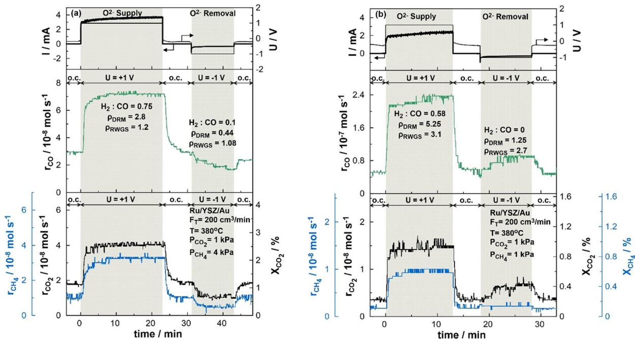
Fig. 8 Transient effect of constant applied positive (+1 V) and negative (-1 V) potential on the catalytic rate of  $CO_2$  and  $CH_4$  consumption (bottom left), conversion of limiting reactant (bottom right), total CO production (middle) and produced current (top left). (a)  $P_{CO_2} = 1$  kPa,  $P_{CH_4} = 4$  kPa (reducing conditions). (b)  $P_{CO_2} = 1$  kPa,  $P_{CH_4} = 1$  kPa (stoichiometric conditions).  $F = 200$   $cm^3$   $min^{-1}$ ,  $T = 380$   $^\circ C$ .
