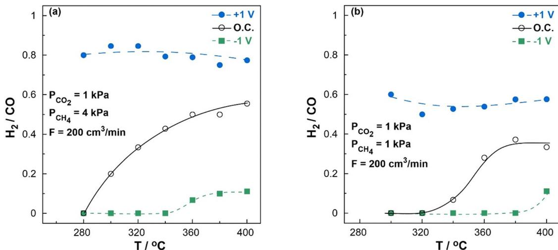
Fig. 6 Steady-state effect of temperature on the  $H_2/CO$  ratio under open-circuit (o.c.), positive polarization ( $U_{WR} = +1$  V) and negative polarization ( $U_{WR} = -1$  V) conditions. (a)  $P_{CO_2} = 1$  kPa,  $P_{CH_4} = 4$  kPa (reducing conditions). (b)  $P_{CO_2} = 1$  kPa,  $P_{CH_4} = 1$  kPa (stoichiometric conditions).  $F = 200$  cm<sup>3</sup> min<sup>-1</sup>.
