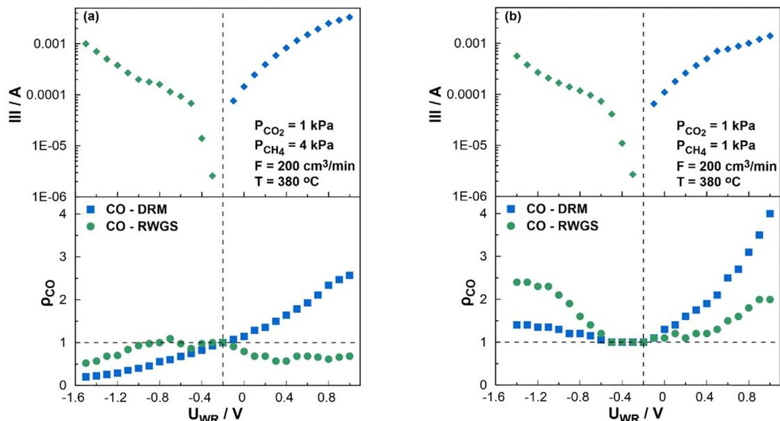
Fig. 10 Steady-state effect of applied potential on the rate enhancement ratio of CO,  $\rho$  (bottom) and the produced current (Tafel plot, top). (a)  $P_{CO_2} = 1$  kPa,  $P_{CH_4} = 4$  kPa (reducing conditions). (b)  $P_{CO_2} = 1$  kPa,  $P_{CH_4} = 1$  kPa (stoichiometric conditions).  $F = 200$  cm<sup>3</sup> min<sup>-1</sup>,  $T = 380$  °C.
