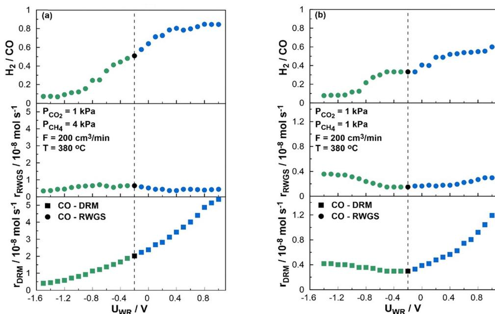
Fig. 9 Steady-state effect of applied potential on the catalytic rate of CO production during the DRM (bottom) and RWGS (middle) reaction and the H<sub>2</sub>/CO ratio (top). (a)  $P_{CO_2} = 1$  kPa,  $P_{CH_4} = 4$  kPa (reducing conditions). (b)  $P_{CO_2} = 1$  kPa,  $P_{CH_4} = 1$  kPa (stoichiometric conditions).  $F = 200 \text{ cm}^3 \text{ min}^{-1}$ ,  $T = 380 \text{ }^\circ\text{C}$ .
