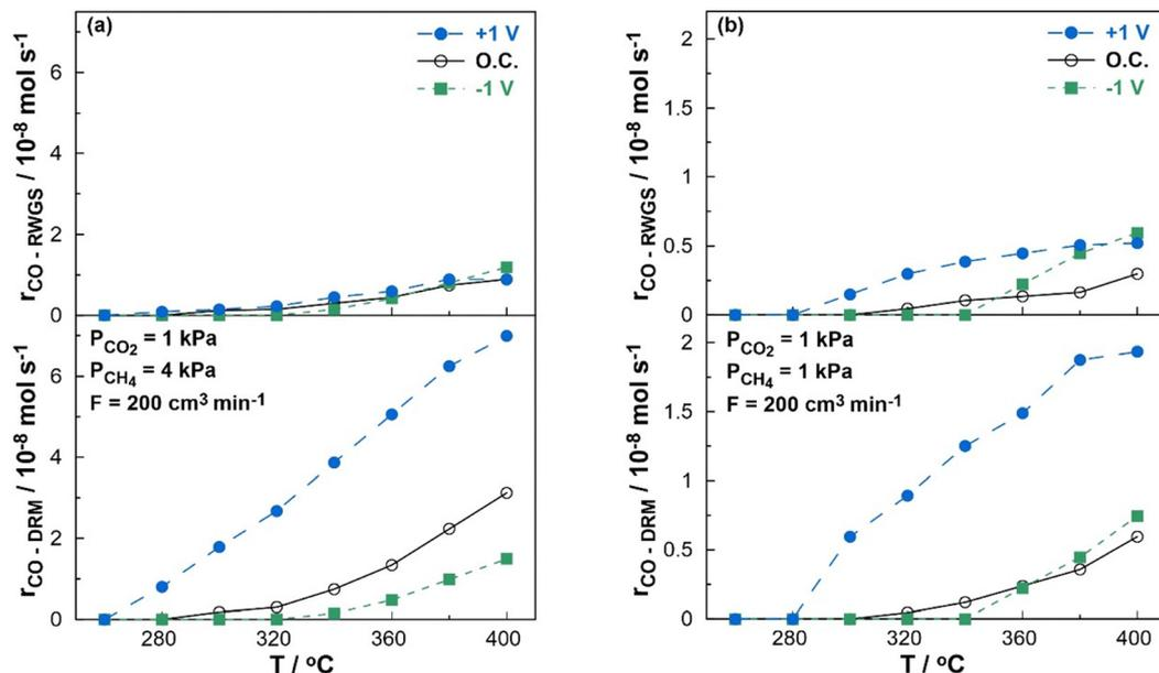
Fig. 5 Steady-state effect of temperature on the catalytic rate of CO production during the DRM reaction (bottom) and RWGS reaction (top) under open-circuit (o.c.), positive polarization ( $U_{WR} = +1$  V) and negative polarization ( $U_{WR} = -1$  V) conditions. (a)  $P_{CO_2} = 1$  kPa,  $P_{CH_4} = 4$  kPa (reducing conditions). (b)  $P_{CO_2} = 1$  kPa,  $P_{CH_4} = 1$  kPa (stoichiometric conditions).  $F = 200$  cm<sup>3</sup> min<sup>-1</sup>.
