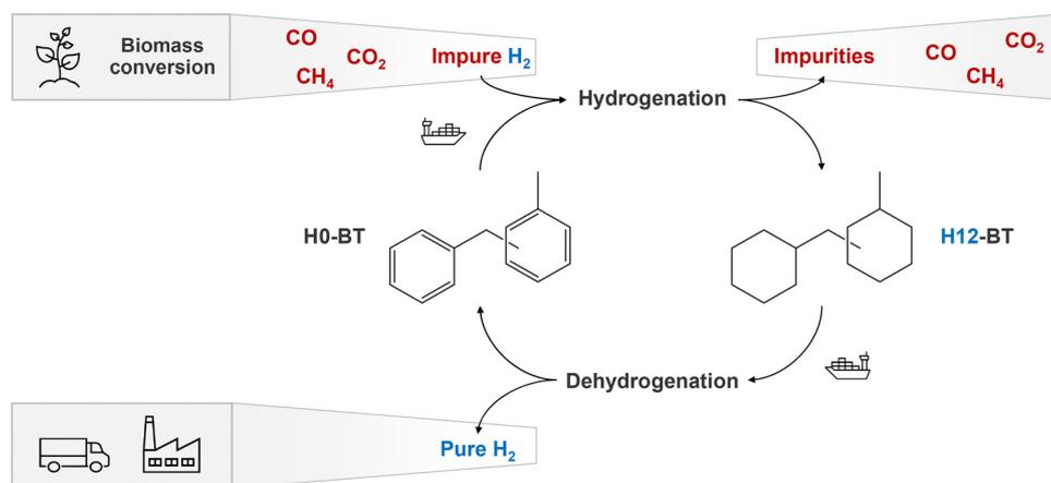
Fig. 1 LOHC hydrogenation with impure hydrogen from biogenic sources allows for chemical hydrogen storage and purification in a single process step.
