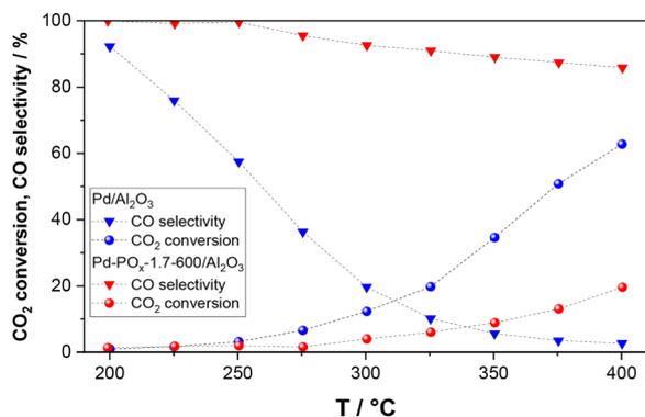
Fig. 5  $CO_2$  conversion and CO selectivity of  $Pd/Al_2O_3$  and  $Pd-PO_x-1.7-600/Al_2O_3$  over temperature during  $CO_2$  hydrogenation with 0.5 g catalyst, a  $H_2 : CO_2$  ratio of 4 : 1 and a GHSV of 2000  $h^{-1}$  (lot 3).
