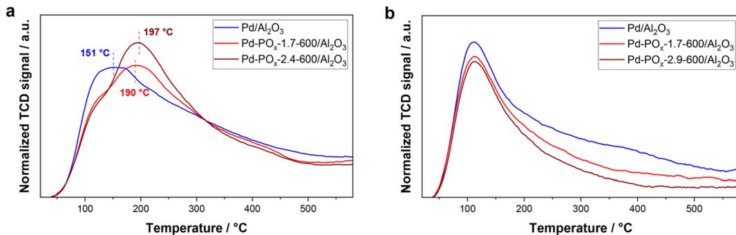
Fig. 10 (a)  $\text{NH}_3$ -TPD of  $\text{Pd}/\text{Al}_2\text{O}_3$  (lot 4),  $\text{Pd-PO}_x\text{-1.7-600}/\text{Al}_2\text{O}_3$  and  $\text{Pd-PO}_x\text{-2.4-600}/\text{Al}_2\text{O}_3$  (lot 2). (b)  $\text{CO}$ -TPD of  $\text{Pd}/\text{Al}_2\text{O}_3$ ,  $\text{Pd-PO}_x\text{-1.7-600}/\text{Al}_2\text{O}_3$  and  $\text{Pd-PO}_x\text{-2.9-600}/\text{Al}_2\text{O}_3$  (lot 2).
