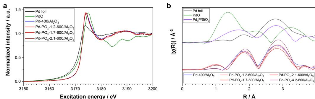
Fig. 8 (a) Normalized Pd L<sub>3</sub>-edge XANES spectra and (b) Fourier-transformed Pd L<sub>2</sub>-edge EXAFS spectra (*k*<sup>2</sup>-weighted, *R*-space) of Pd foil, PdO, Pd-400/Al<sub>2</sub>O<sub>3</sub>, Pd-PO<sub>x</sub>-1.2-600/Al<sub>2</sub>O<sub>3</sub>, Pd-PO<sub>x</sub>-1.7-600/Al<sub>2</sub>O<sub>3</sub>, Pd-PO<sub>x</sub>-2.1-600/Al<sub>2</sub>O<sub>3</sub> and Pd-PO<sub>x</sub>-4.2-600/Al<sub>2</sub>O<sub>3</sub> (lot 2).
