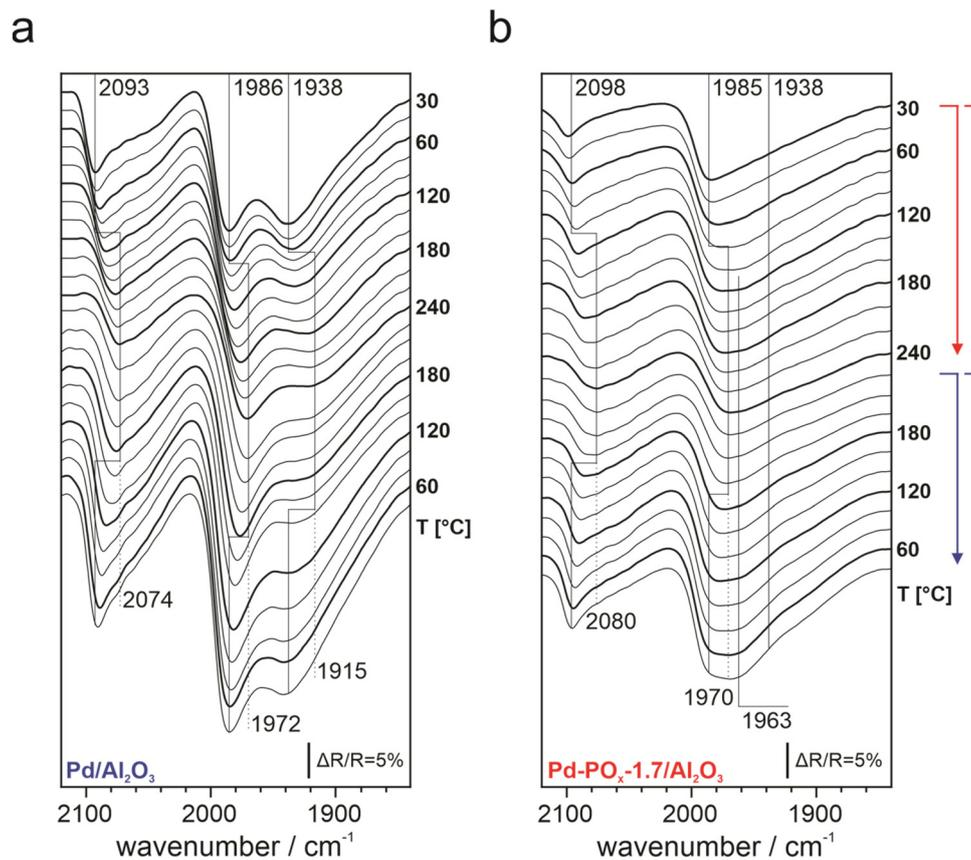
Fig. 11 CO-DRIFT spectra recorded during temperature-programmed experiments with (a) Pd/Al<sub>2</sub>O<sub>3</sub> and (b) Pd-PO<sub>x</sub>-1.7-600/Al<sub>2</sub>O<sub>3</sub> (lot 3).
