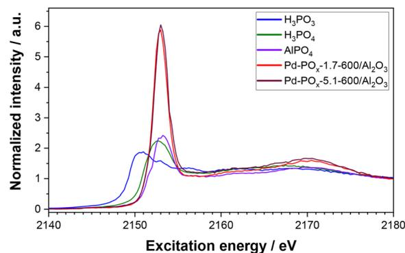
**Fig. 9** Normalized P K-edge XANES spectra of H<sub>3</sub>PO<sub>3</sub>, H<sub>3</sub>PO<sub>4</sub>, AlPO<sub>4</sub>, Pd-PO<sub>x</sub>-1.7-600/Al<sub>2</sub>O<sub>3</sub> and Pd-PO<sub>x</sub>-5.1-600/Al<sub>2</sub>O<sub>3</sub> (lot 2).
