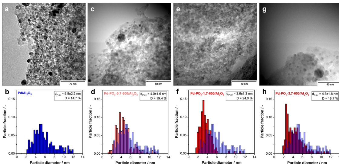
Fig. 7 HR-TEM and particle size distribution of (a) and (b) Pd/Al<sub>2</sub>O<sub>3</sub>, (c) and (d) Pd-PO<sub>x</sub>-0.7-600/Al<sub>2</sub>O<sub>3</sub>, (e) and (f) Pd-PO<sub>x</sub>-1.7-600/Al<sub>2</sub>O<sub>3</sub> and (g) and (h) Pd-PO<sub>x</sub>-3.7-600/Al<sub>2</sub>O<sub>3</sub> (all lot 1).
