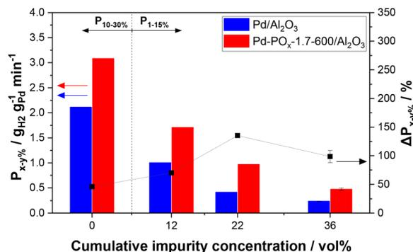
Fig. 4 H0-BT hydrogenation with  $H_2$ /mixed at 240 °C and 30 bar  $H_2$ -pressure.  $P_{x-y\%}$  and  $\Delta P_{x-y\%}$  of  $Pd/Al_2O_3$  and  $Pd-PO_x-1.7-600/Al_2O_3$  ( $n_P : n_{Pd} = 1.7 \pm 0.3$ ) with  $n_{Pd} : n_{H_0-BT} = 4.1 \times 10^{-4}$  (lot 2).
