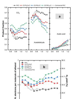
Fig. 8 (a) Product distribution for the different electrocatalysts at different cell voltages, and (b) number of electrons per molecule of ethanol and faradaic efficiency as a function of the cell voltage.
