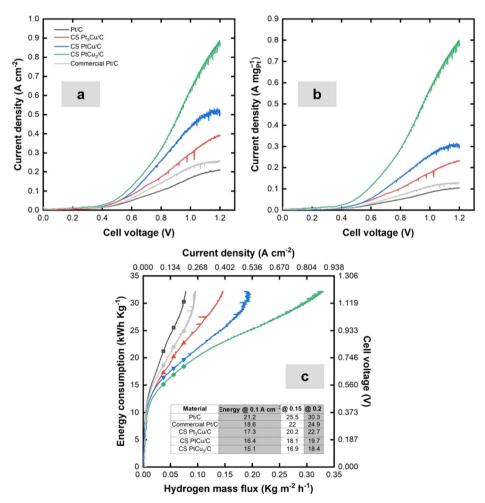
Fig. 7 Electrolysis curves for the high-temperature DEPEME at 150 °C based on: (a) electrode active area, (b) Pt mass; (c) energy requirements as a function of the  $H_2$  produced (inset table: energy required (kWh  $K_2^{-1}$   $H_2$ ) at 0.1, 0.15, and 0.2 A cm<sup>-2</sup>).
