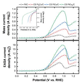
Fig. 6 EEO curves in the anodic scans (5 mV s $^{-1}$ ) in 1 mol L $^{-1}$  H $_3$ PO $_4$  and 5 mol L $^{-1}$  ethanol for the different electrocatalysts.
