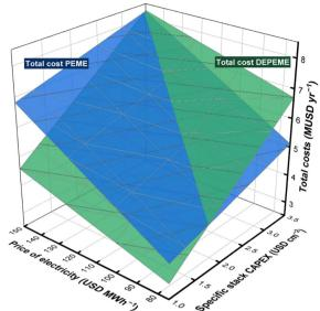
Fig. 9 Evolution of the total costs depending on the price of electricity and specific stack CAPEX.
