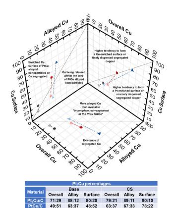
Fig. 3 Projections of the Cu atomic percentages on the surface (XPS), in the PtCu alloy (XRD), and the overall (ICP-OES) ( $\bullet \circ : Pt_3Cu/C; \blacksquare : PtCu/C; \triangle : PtCu_3/C; light symbols correspond to CS materials). The inset table collects the corresponding percentages for each analysis.$
