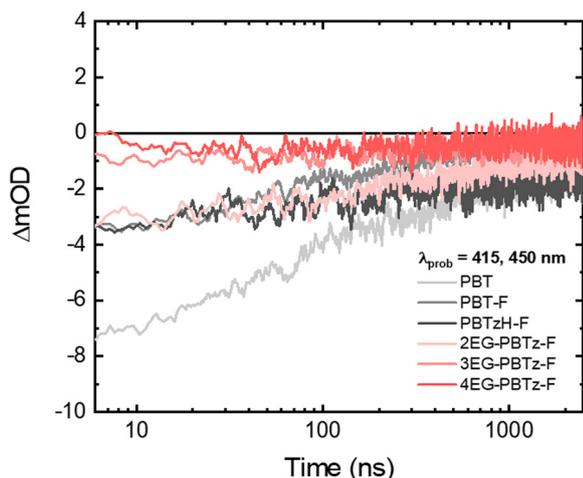
Fig. 5 TA kinetics of polymer particle dispersion. All polymers were dispersed in the same volume ratio of TEA:MeOH:H<sub>2</sub>O and probed at 415 or 450 nm.
