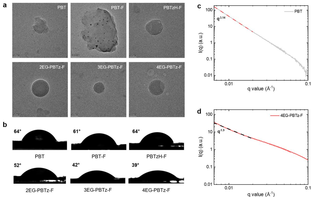
Fig. 6 Morphology and hydrophilicity measurements of the polymers. (a) Transmission electron microscopy (TEM) image of polymer dispersion in the same volume ratio of TEA:MeOH:H<sub>2</sub>O. (b) Water contact angle of the polymers in pellets. Small-angle X-ray scattering (SAXS) profiles of (c) **PBT** and (d) **4EG-PBTz-F** obtained from the polymer dispersions prepared in a TEA:MeOH:H<sub>2</sub>O solvent with the same volume ratio.
