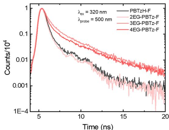
**Fig. 3** Time-resolved photoluminescence (Tr-PL) decays of dispersion of polymer particles (**PBTzH-F**, **2EG-PBTz-F**, **3EG-PBTz-F** and **4EG-PBTz-F**). All polymers were dispersed in the same volume ratio of TEA:MeOH:H<sub>2</sub>O, excited at 320 nm, and probed at 500 nm using the time-correlated single photon counting method.
