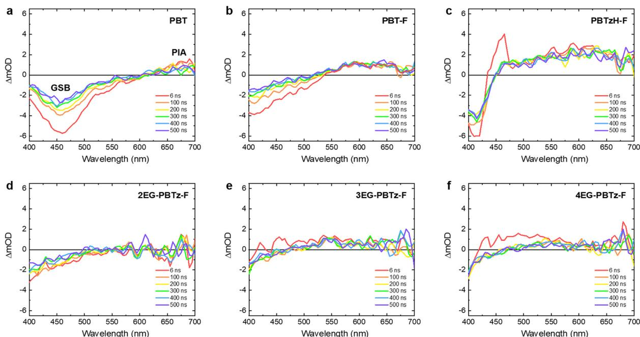
Fig. 4 Transient absorption (TA) spectra of the polymer nanoparticle dispersion of (a) **PBT**, (b) **PBT-F**, (c) **PBTzH-F**, (d) **2EG-PBTz-F**, (e) **3EG-PBTz-F**, and (f) **4EG-PBTz-F**. All polymers were dispersed in the same volume ratio of TEA:MeOH:H<sub>2</sub>O and measured at various nanosecond timescale delays with 355 nm excitation ( $2 \text{ mJ cm}^{-2}$ ).
