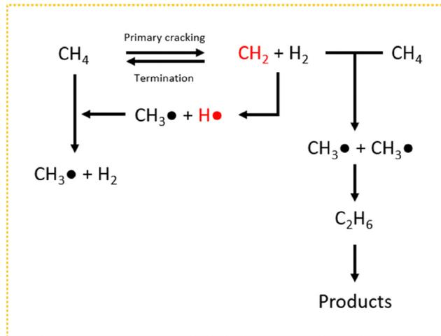
Fig. 6 Non-catalytic methane decomposition reaction mechanism where primary rupture to  $CH_2$  and  $H_2$  is the rate-determining step.<sup>110,111</sup>
