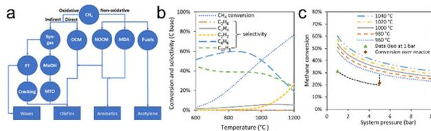
**Fig. 3** (a) Converting methane to C<sub>2+</sub> hydrocarbons *via* different conversion strategies, and (b) thermodynamic equilibrium methane conversion, C<sub>2+</sub> product selectivity and (c) methane conversion at thermodynamic equilibrium as a function of reactor pressure for NOCM under thermal conditions are calculated using Aspen Plus<sup>89</sup> (MDA: methane dehydroaromatization). Reprinted with permission from ref. 17 Copyright 2021 American Chemical Society.
