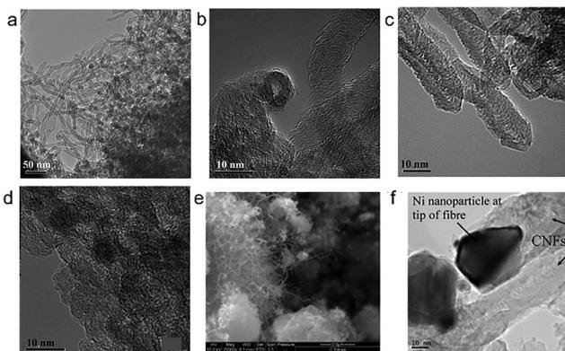
Fig. 8 TEM images of the carbon nanofibers produced at 500 °C using plasma-treated Ni/Al<sub>2</sub>O<sub>3</sub>, where (a) base-growth CNFs, (b) open tip CNFs, (c) closed tip CNFs, and (d) onion-like carbon formation. Reproduced with permission from ref. 135 Copyright 2008 Elsevier. (e) SEM and (f) TEM images of the produced CNFs from DBD plasma-assisted methane decomposition using Ni/Al<sub>2</sub>O<sub>3</sub>. Reproduced with permission from ref. 141 Copyright 2011 Elsevier.
