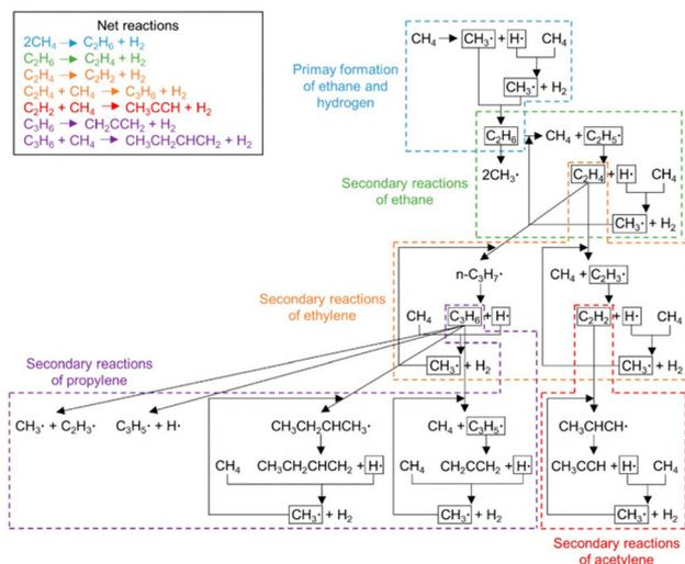
Fig. 5 The reaction mechanism of uncatalyzed methane decomposition as proposed by Chen *et al.*<sup>109</sup> Reproduced with permission from ref. 14 Copyright 2021 American Chemical Society.
