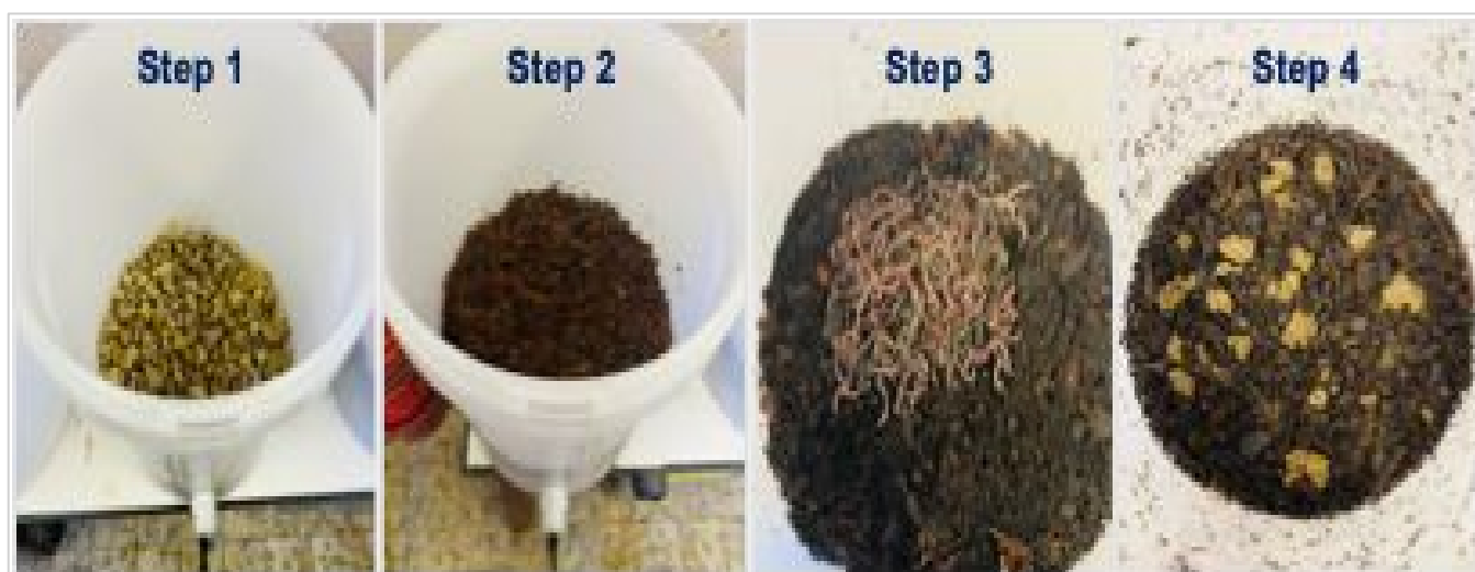
Figure 1: Sequential stages in the setup of the laboratory-scale biodigesters. Shown from left to right: (Step 1) placement of a gravel layer at the base of the container, (Step 2) addition of a coir layer above the gravel, (Step 3) topping up tiger worms above the coir, and (Step 4) daily feeding of pig faeces.
