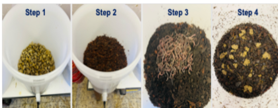
Fig. 1 Sequential stages in the setup of the laboratory-scale biodigesters. Shown from left to right: (step 1) placement of a gravel layer at the base of the container, (step 2) addition of a coir layer above the gravel, (step 3) topping up tiger worms above the coir, and (step 4) daily feeding of pig faeces.
