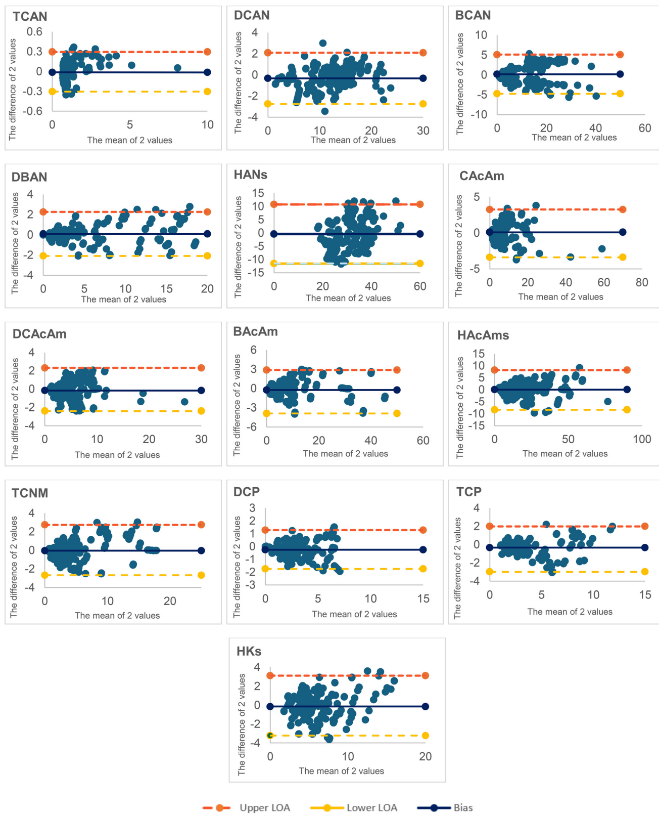
Fig. 4 Bland-Altman plots for the evaluation of the agreement between experimentally determined concentrations and values calculated based on linear models. The mean difference line represents the average bias between the two methods, while the upper and lower LOA are the limits of agreement (LOA) (mean difference \pm 1.96 \times standard deviation). Approximately 95% of data points should fall between these upper and lower limits to have a good agreement.
